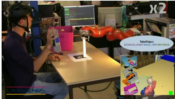
Figure 11: The face-to-face setup of the Clean the Table study. The physical situation, the SPARK model, and the current step of the plan are visible on the picture.
