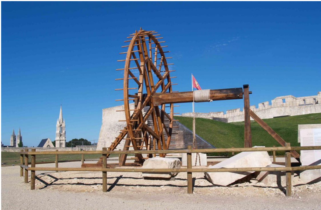
Fig. 14- Winch used to bring to the surface heavy blocks of Pierre de Caen from underground quarries - note the white colour of the stone © D. Peeters
