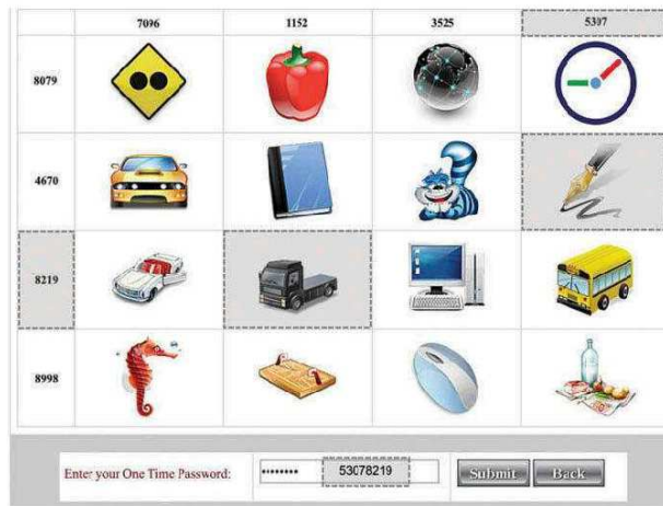
Figure 2. GOTPass image recognition and OTP code entry – Assuming security-level option 3 is in use (top axis for the first pass-image + left axis for the second pass-image).
