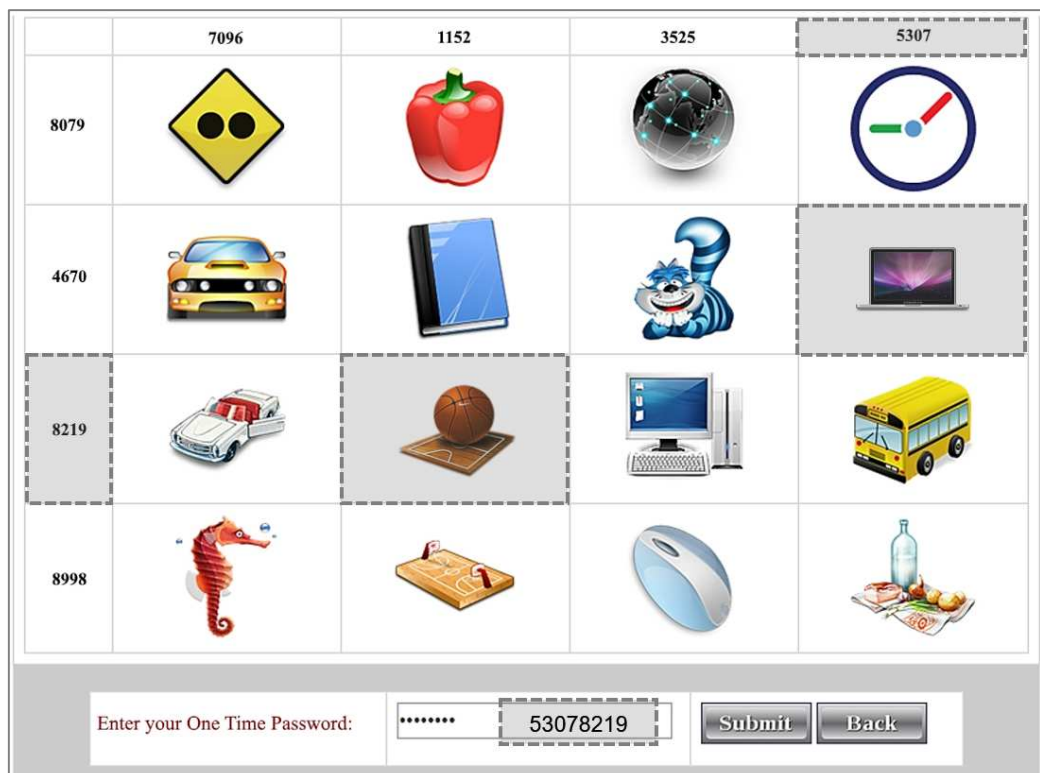
Figure 5-11: GOTPass image recognition and OTP code entry Assuming security level option 3 is in use (top axis code for the first pass-image + left axis code for the second pass-image)
