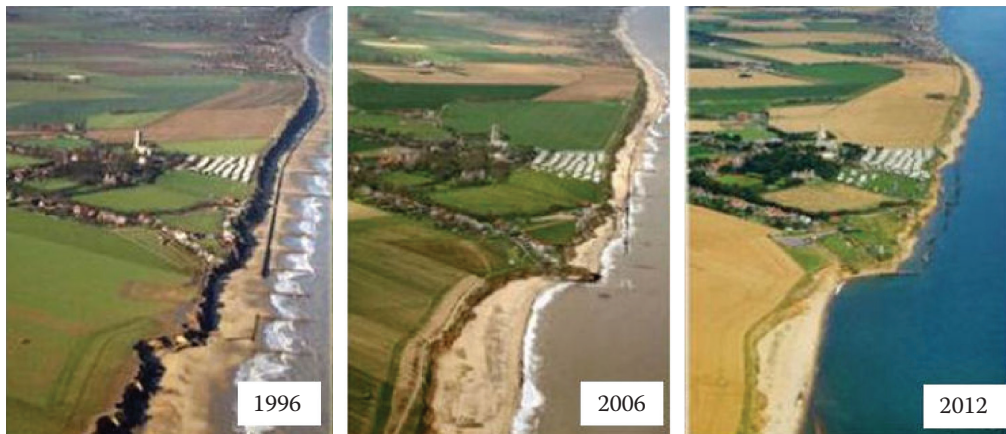
Figure 3 The eroding coastline at Happisburgh, Norfolk, United Kingdom. The removal of the groynes in 1991 led to severe coastal erosion and a landward retreat of about 100 m. (Photos copyright Mike Page.)
