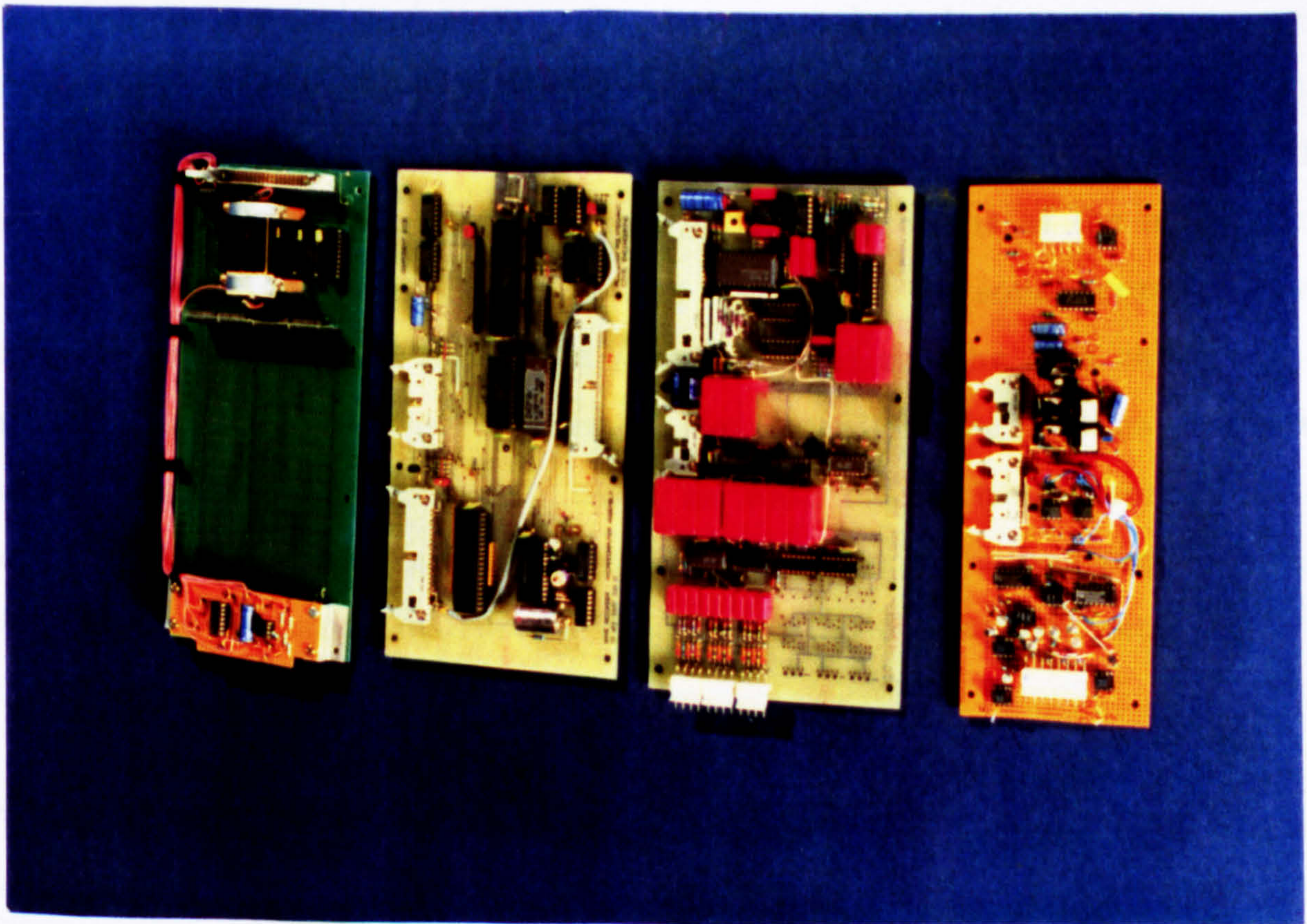
Plate 3 : The four main circuit board assemblies. From the left: data store, microcomputer, signal conditioning, and power supply.
