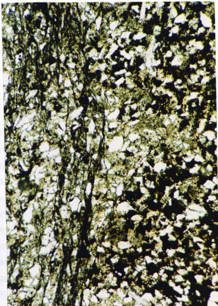
Plate 4.21 Photomicrograph (x64) of the quartz (right) and phyllosilicate (left) domains produced during the formation of the first phase cleavage; plane polarised light. Renney Rocks Formation, Heybrook Bay [SX 4965 4870].
