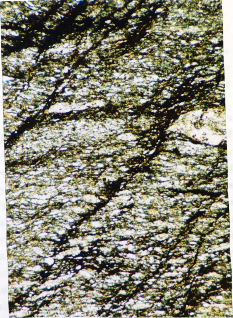
Plate 4.25 Photomicrograph (x64) of the crenulation cleavage, plane polarised light. Bovisand Formation, Crownhill Bay [SX 4925 5025].
