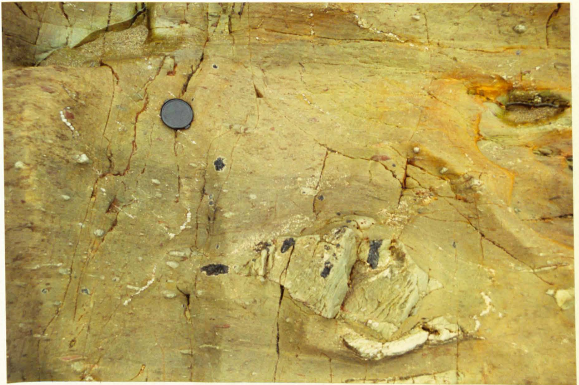
Plate 3.14 Paraconglomerate containing sedimentary and volcanic clasts within the Yealm Formation; Erme Estuary [SX 6180 4740].
