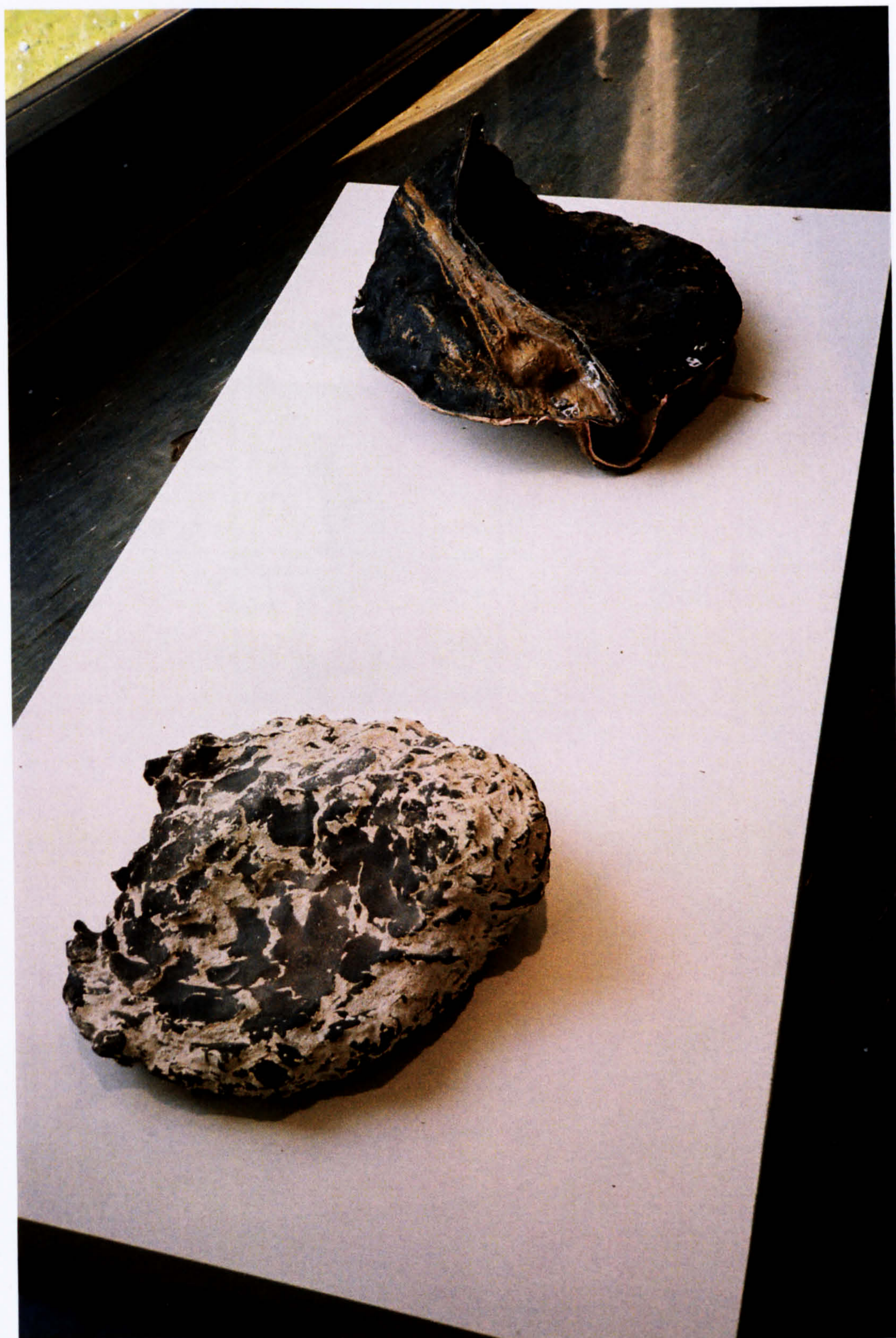
XLII. Failed Shell Cast and Fibreglass Case for Wax in Rubber Mould. Pl.183 x 91 x 10cm
