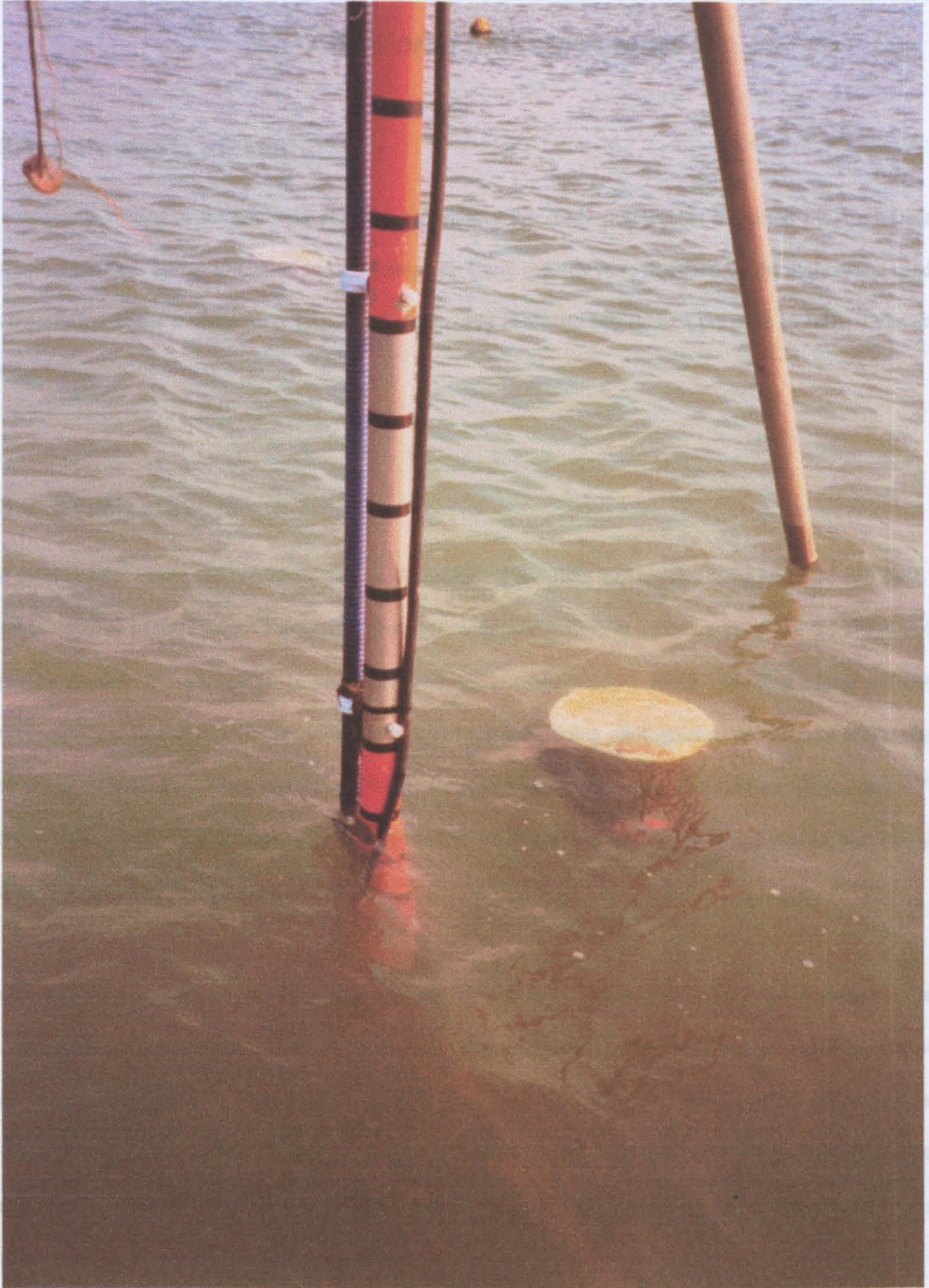
Figure 3-4 Visual wave staff, resistance staff and pressure transducer during the equipment inter-comparison.
