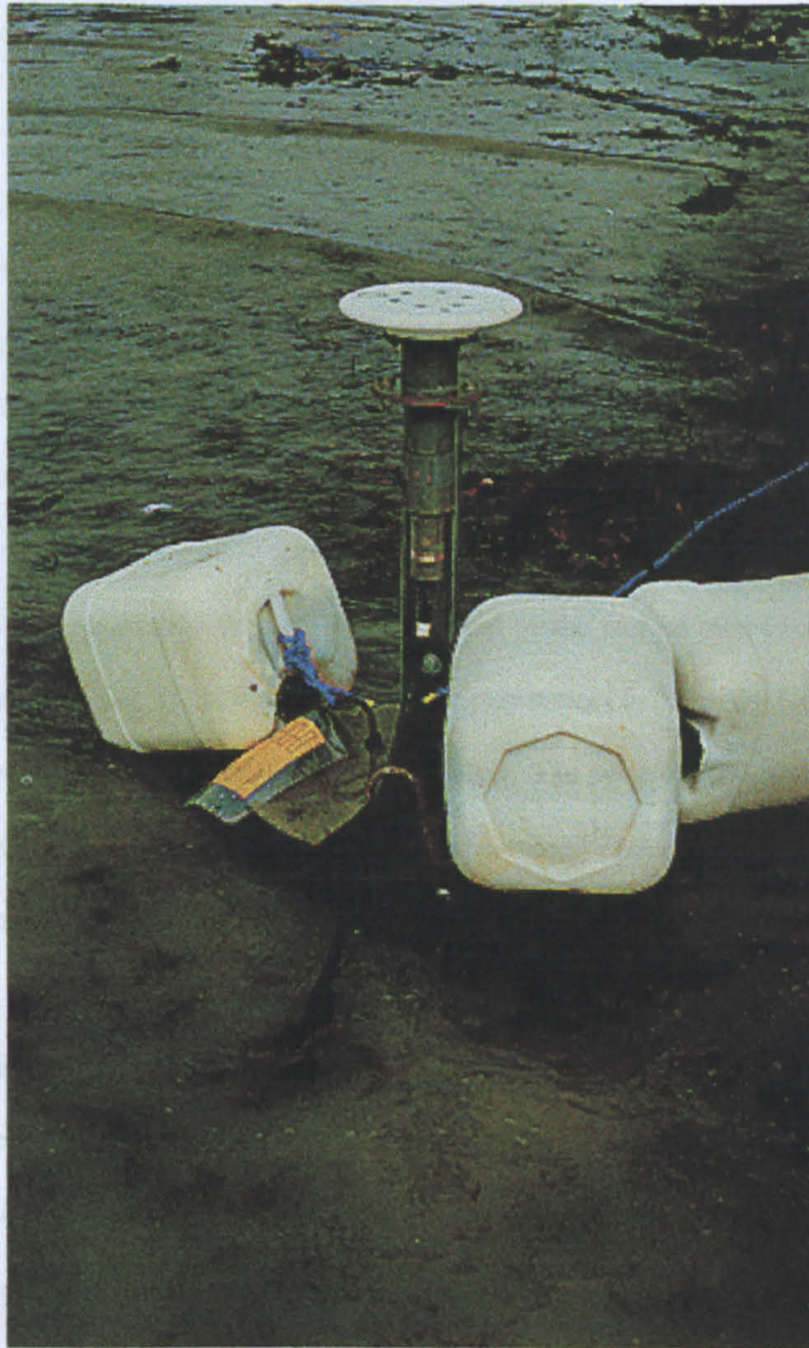
Figure 3-3 Wave recorder transducer with floats attached ready for deployment.
