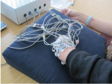
Fig. 2. The surface electrodes locations for the amputees showing the left stump for CGI.
