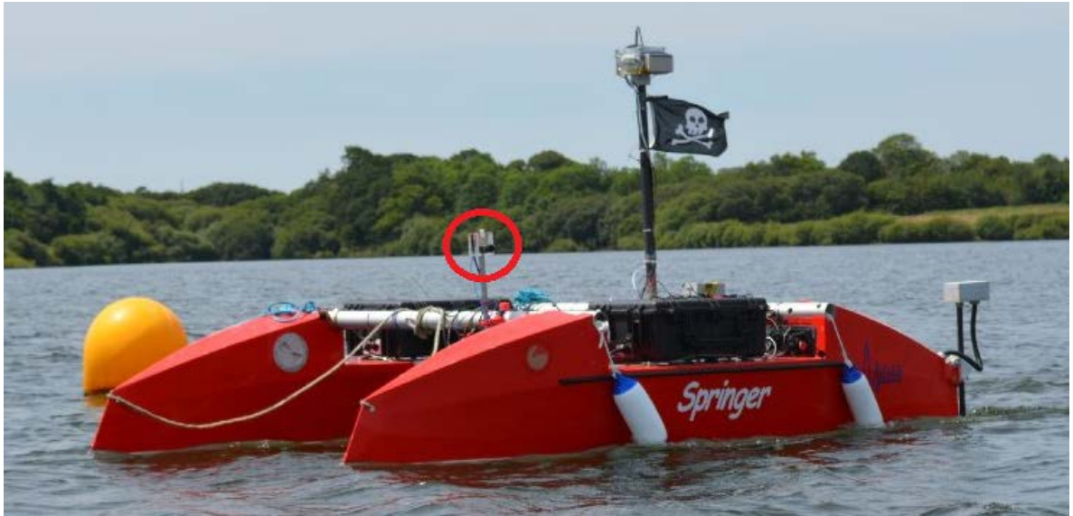
Figure 1.1. The unmanned surface vehicle known as “Springer”. The camera (circled in red) is mounted on the left hull, pointing sideways.
