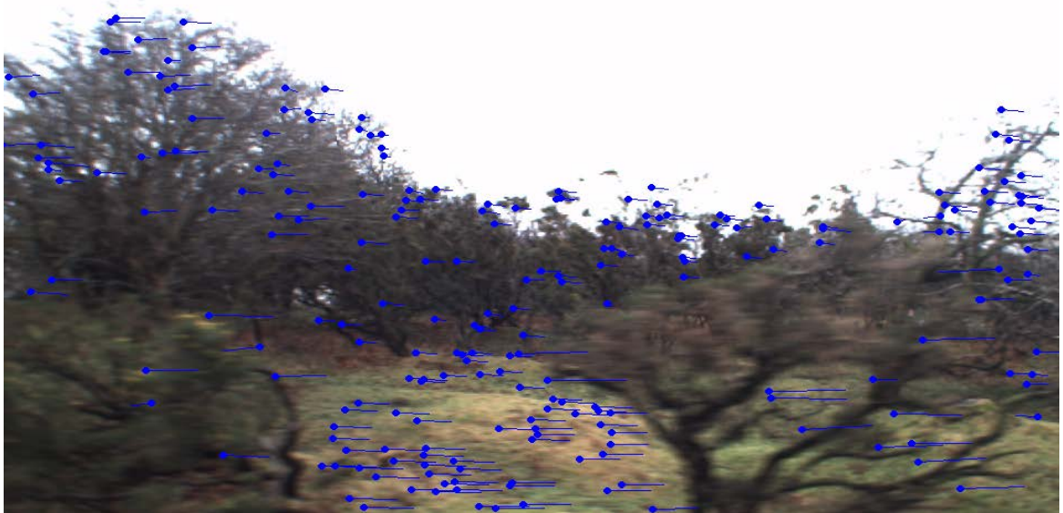
Figure 5.8. The remaining optical flow following removal of outliers inconsistent with the RANSAC/MCMC based computation of the fundamental matrix.
