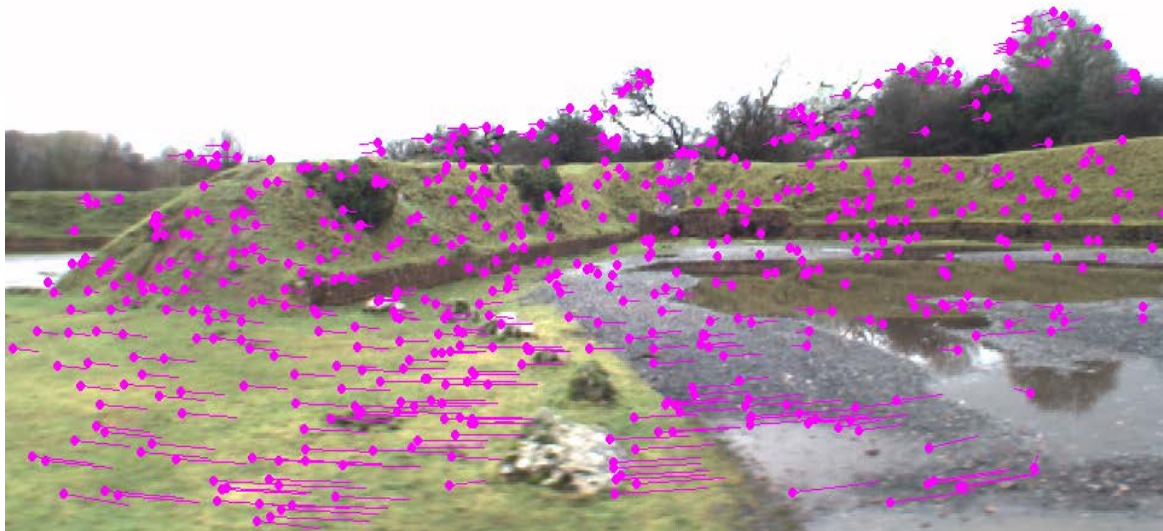
Figure 2.8. Sparse optical flow vectors between the 1st and 6th frame of the sequence estimated using the pyramidal LK tracker.
