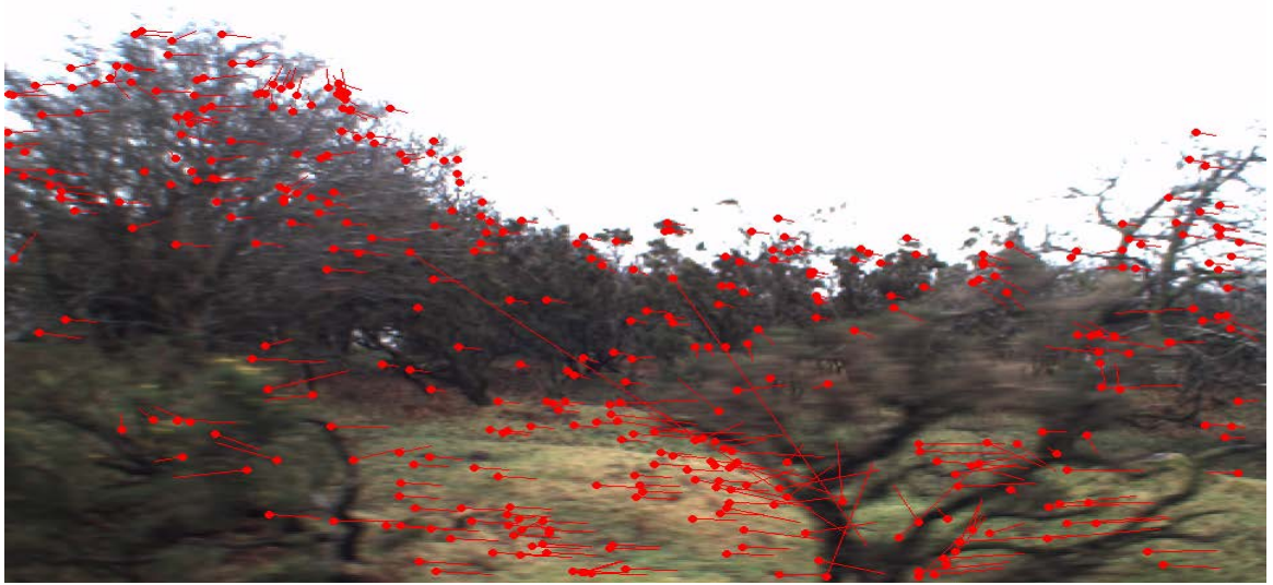
Figure 5.7. The optical flow vectors after the removal of unsuccessfully tracked features according to the LK tracker.
