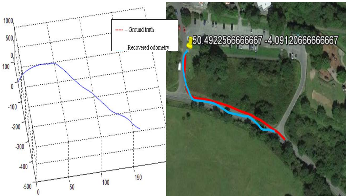
Figure 6.9. Relative pose odometry from a ride in countryside residential areas (0.6 km). Plot scale on the left is arbitrary and therefore axes do not represent actual length units.
