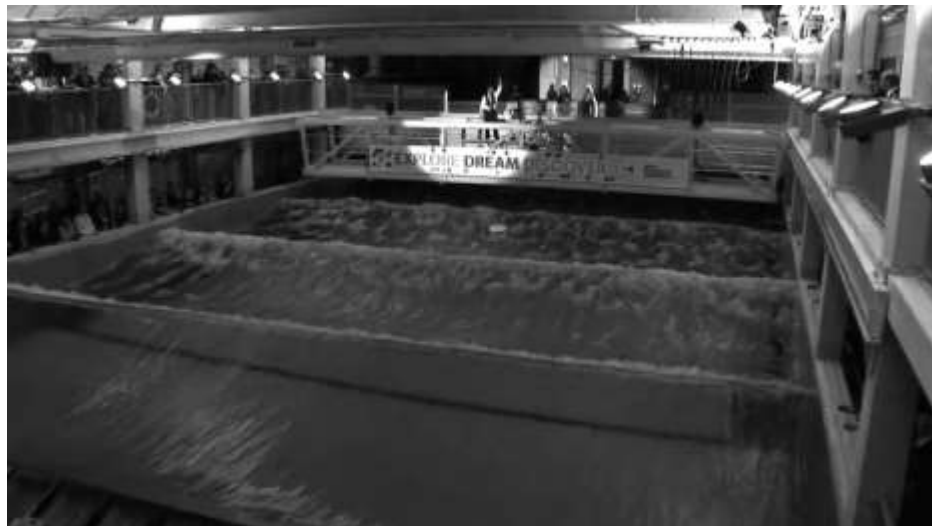
Fig. 3. Over-driven Sine wave during demonstration; the demonstrator can be seen in spotlight on the bridge-like gantry, and the buoy in the water below.
