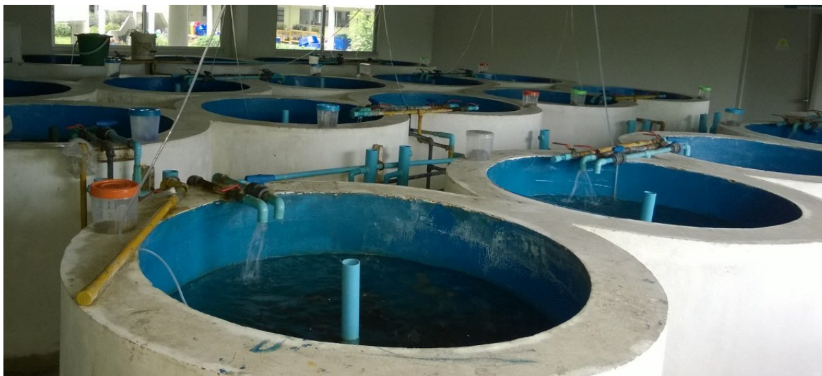
Figure 4.1: Flow-through system (FS) at the Division of Animal Production Technology and Fisheries, KMITL where tilapia were held during the trial. The experimental system consisted of circular concrete tanks with a capacity of 580 L. Water was sourced from the local river system and was monitored daily (pH, DO and temperature) and weekly (nitrogen wastes – ammonia, nitrite, nitrate) to ensure appropriate conditions for tilapia.
