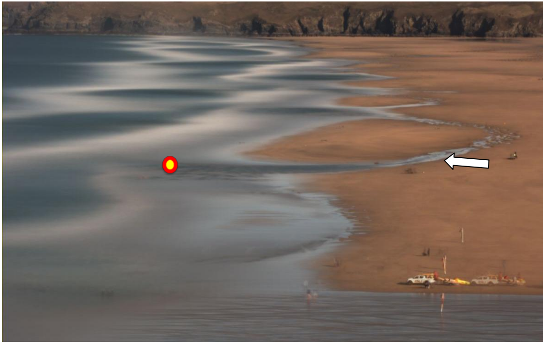
Figure 3: Time averaged image of bar-rip morphology at Perranporth beach (arrow marks rip system used in study; circle marks position of instrumentation).
