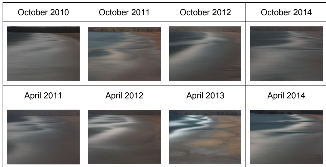
Figure 7.5: ARGUS images captured at low tide showing low tide morphology at Perranporth during STIR 1 (October, 2011) and STIR 2 (April 2013) and for three other years during the same months.
