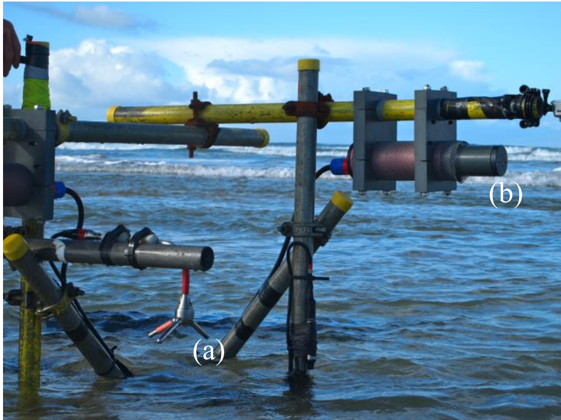
Figure 4: Rig design and position of instruments; (a) ADV head, (b) SRP. The picture was taken at low tide; at mid and high tide the rig is completely submerged.
