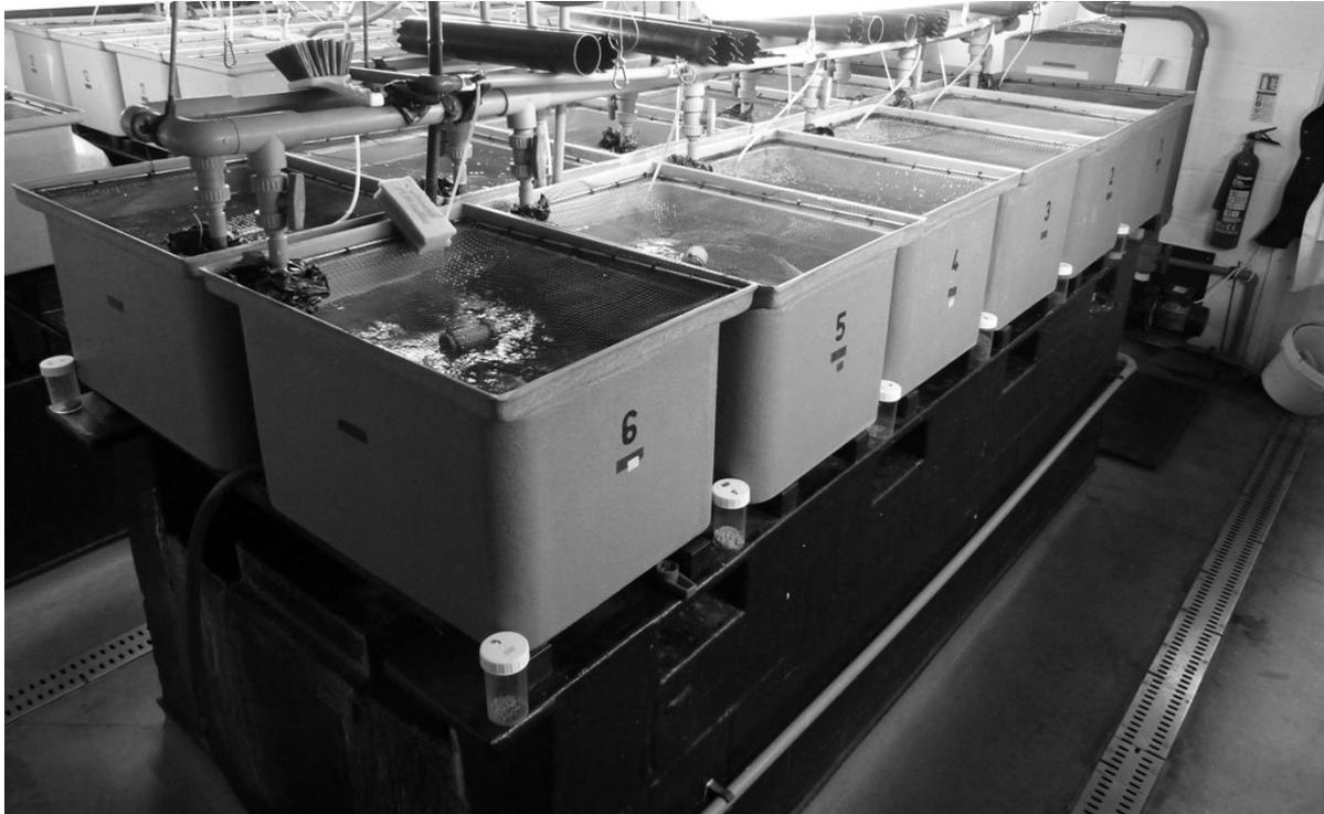
**Plate 7.1** Warmwater RAS utilised for experimental work under Chapter 3, using Nile tilapia.
