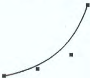
Figure 5.2 Example Bezier curve showing the 4 control points.
