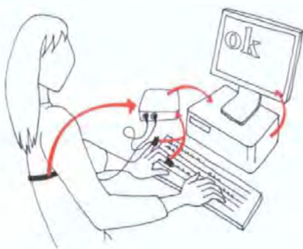
Figure 5.1 Data of a user's breath rate is gathered by the ProComp+ chest band. Data of a user's galvanic skin response and heart rate are gathered from sensors attached to the user's fingers by Velcro. This data is input to the ProComp+ box, and transferred to the computer. The incoming data changes the appearance of each letterform, as the user types. The effects on users of seeing a visualization of their changing physiological states via the morphing of typographic forms is an open-ended question. However, many users said that they get "caught" in "feedback loops," especially regarding heart rate.
