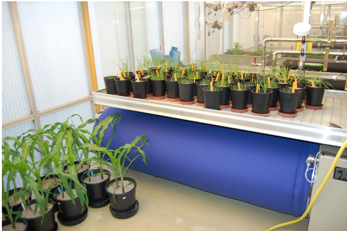
Figure 56 The experimental setup with cooling system. Photo: J. Schläpfer ETHZ 2011
