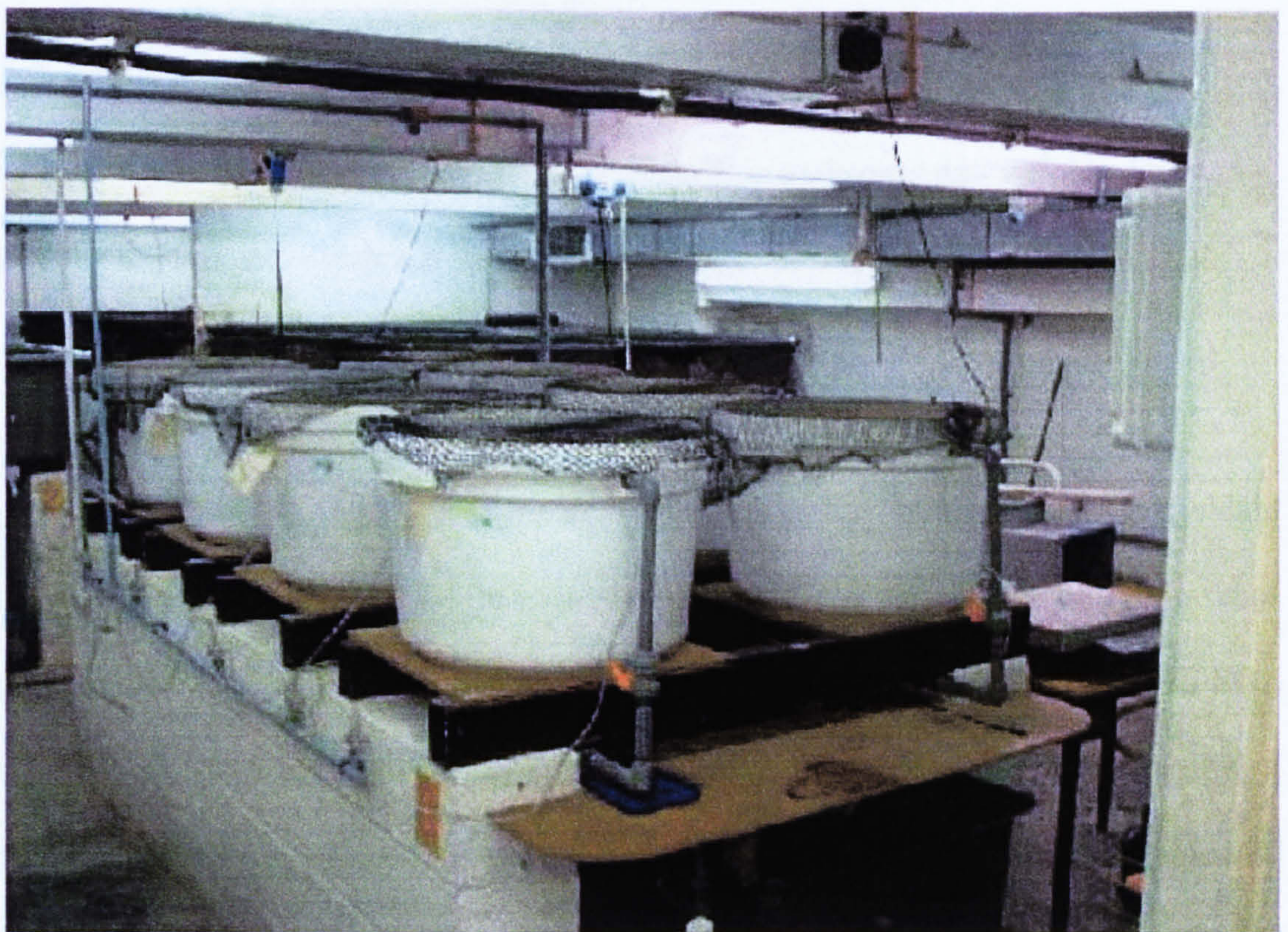
Figure 2.3 photograph of main recirculation system used for the fish feeding and digestibility trials.
