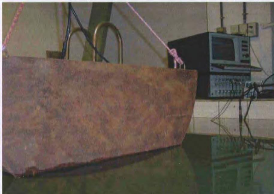
Figure 6.3 Experimental arrangement for underwater acoustic radiation measurement
