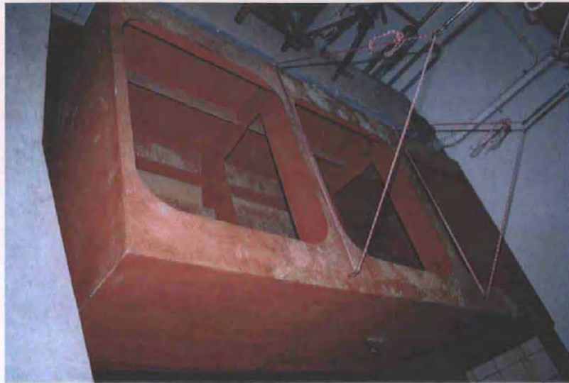
Figure 5.6 The hanging arrangement of the scale engine room model (I)
