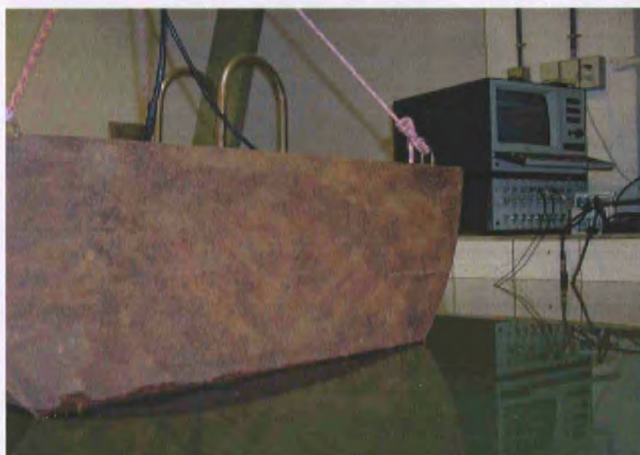
Figure 6.3 Experimental arrangement for underwater acoustic radiation measurement
