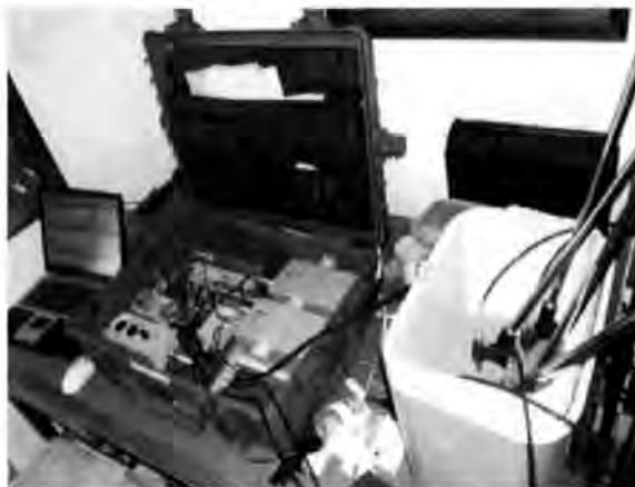
Figure 1: experimental thermal probe measurement kit (during calibration phase, measuring agar immobilised water)
