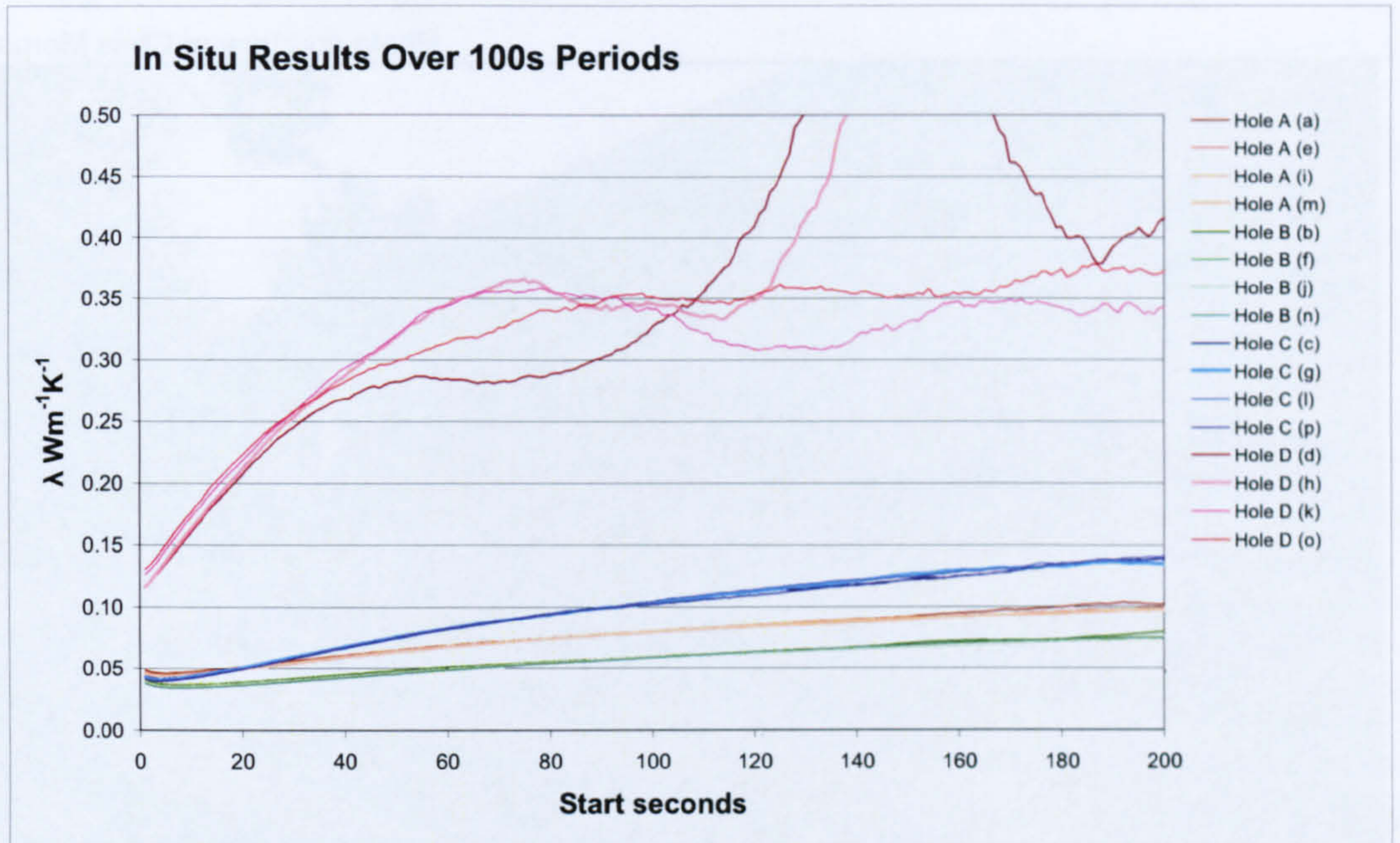
Chart 52: In situ results for clay straw wall construction
