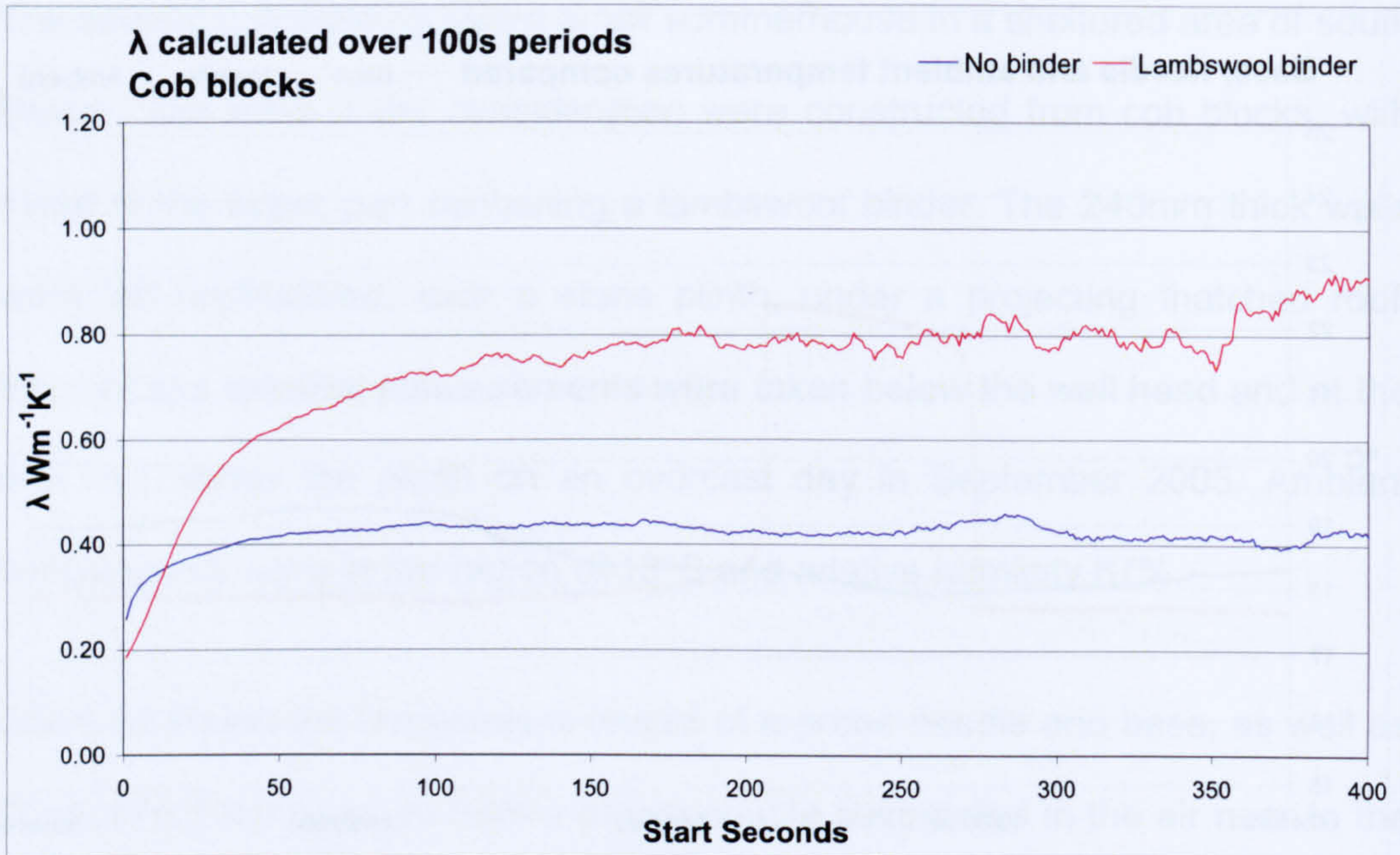
Chart 46: Thermal conductivity, cob blocks with and without lambswool binder
