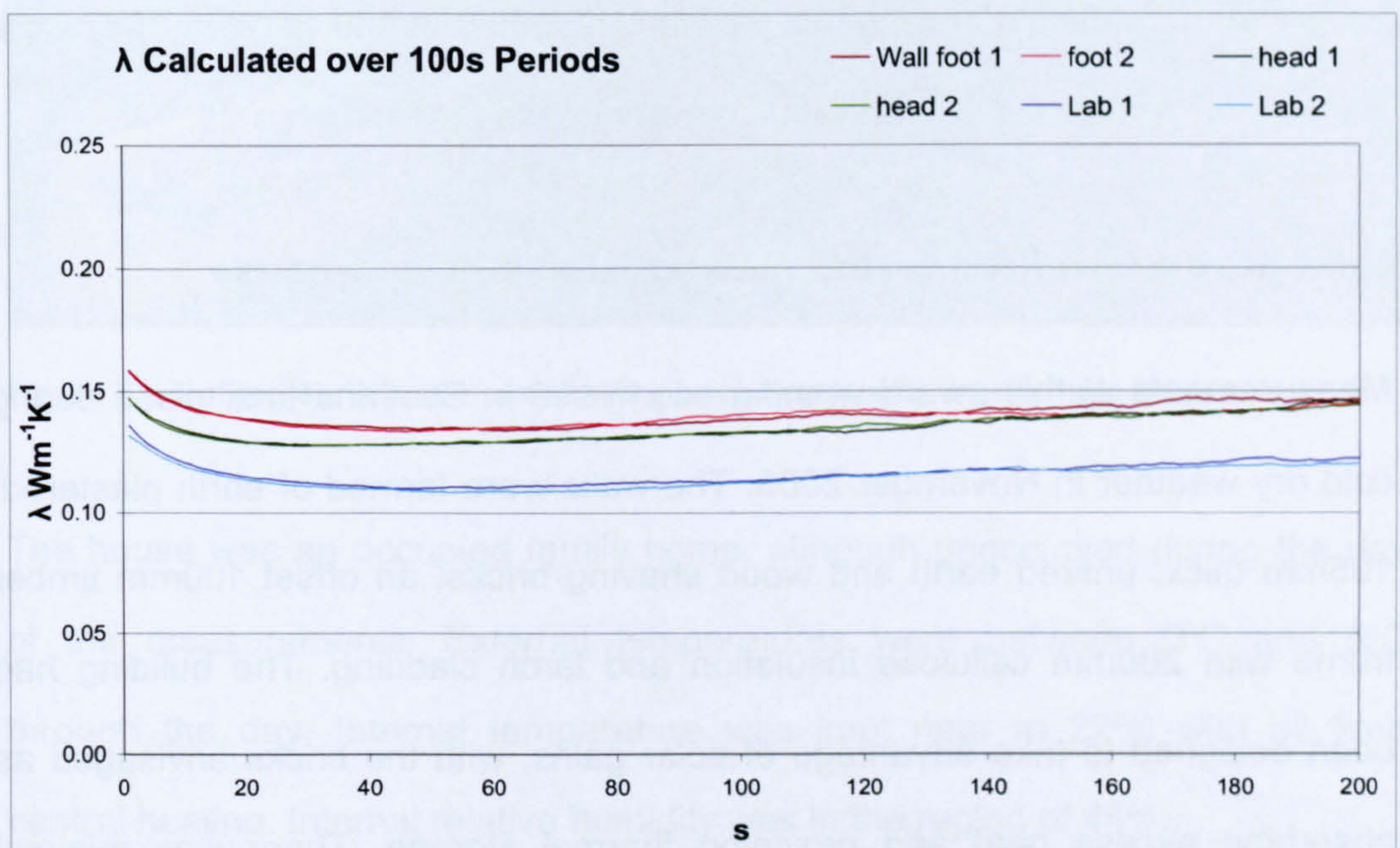
Chart 49: Thermal conductivity, aerated concrete in situ and laboratory results
