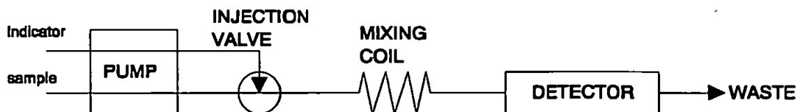
Figure 4.10. Schematic flow diagram of the spectrophotometric pH system used to characterise the reproducibility of the peristaltic pump.
