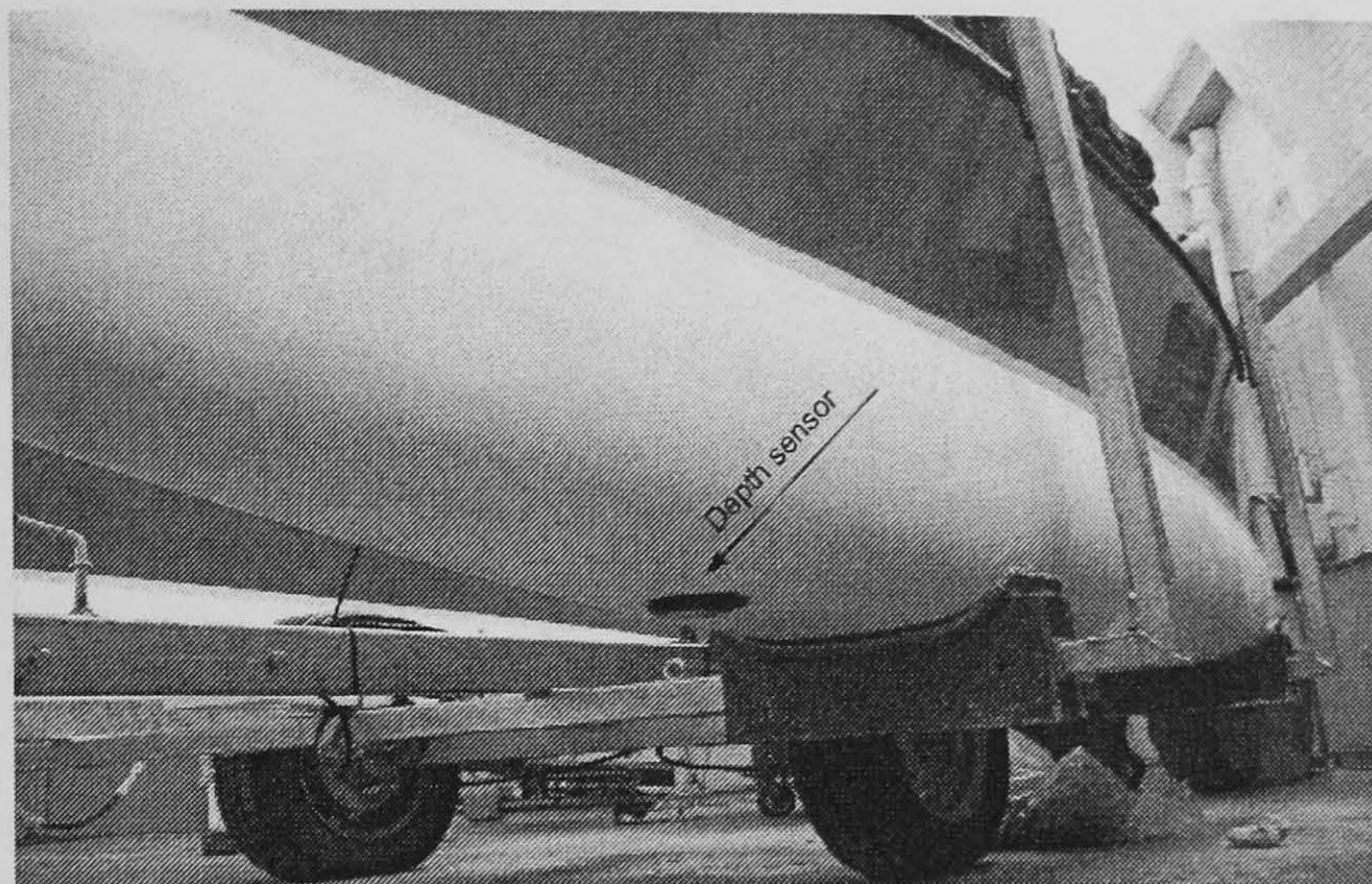
Figure 3.5: Depth sensor at the bottom of the hull
