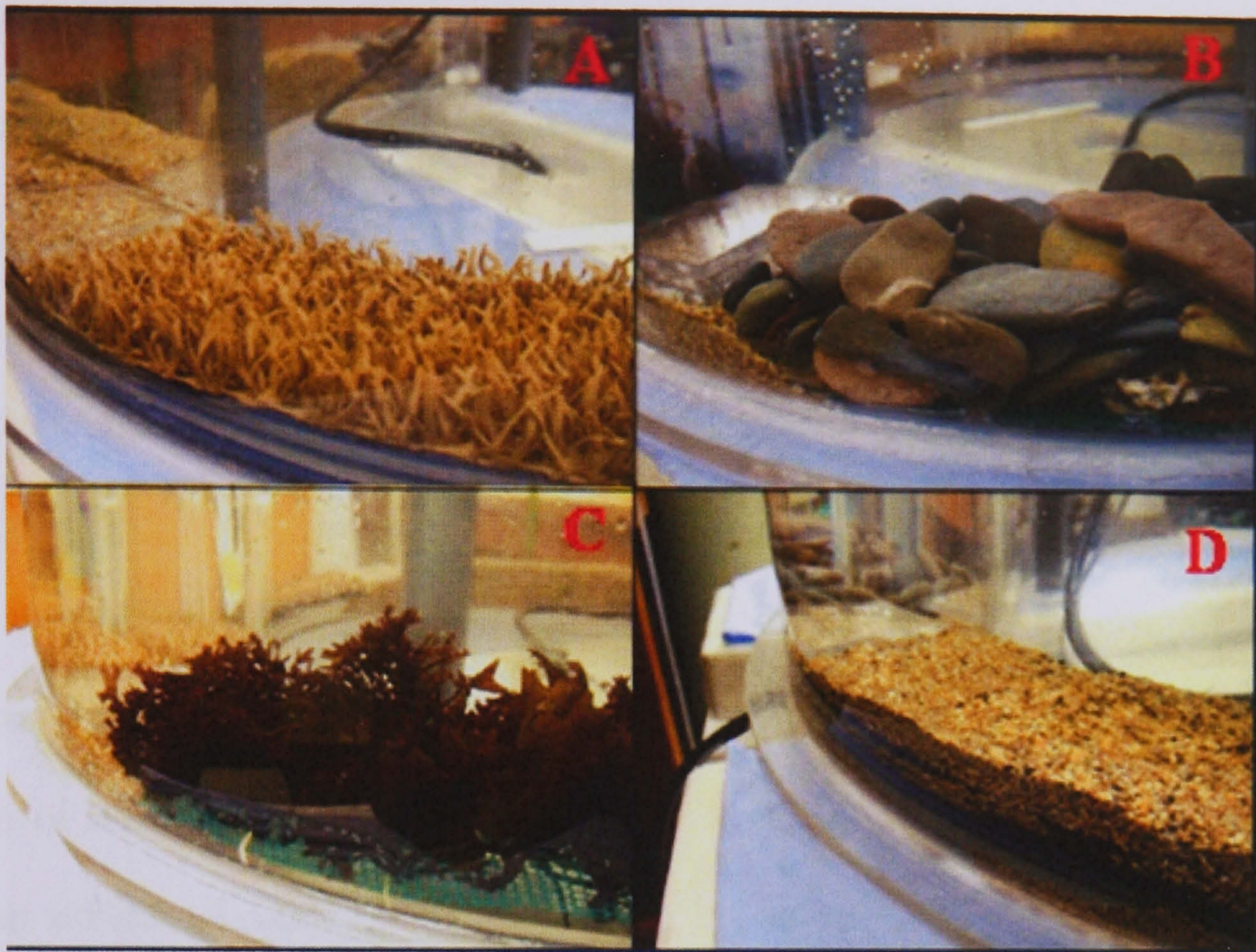
Figure 4.4 Substrata used in the flume experiments: (A) AstroTurf; (B) pebble; (C) red macroalgae, Mastocarpus stellatus ; and (D) sand.
