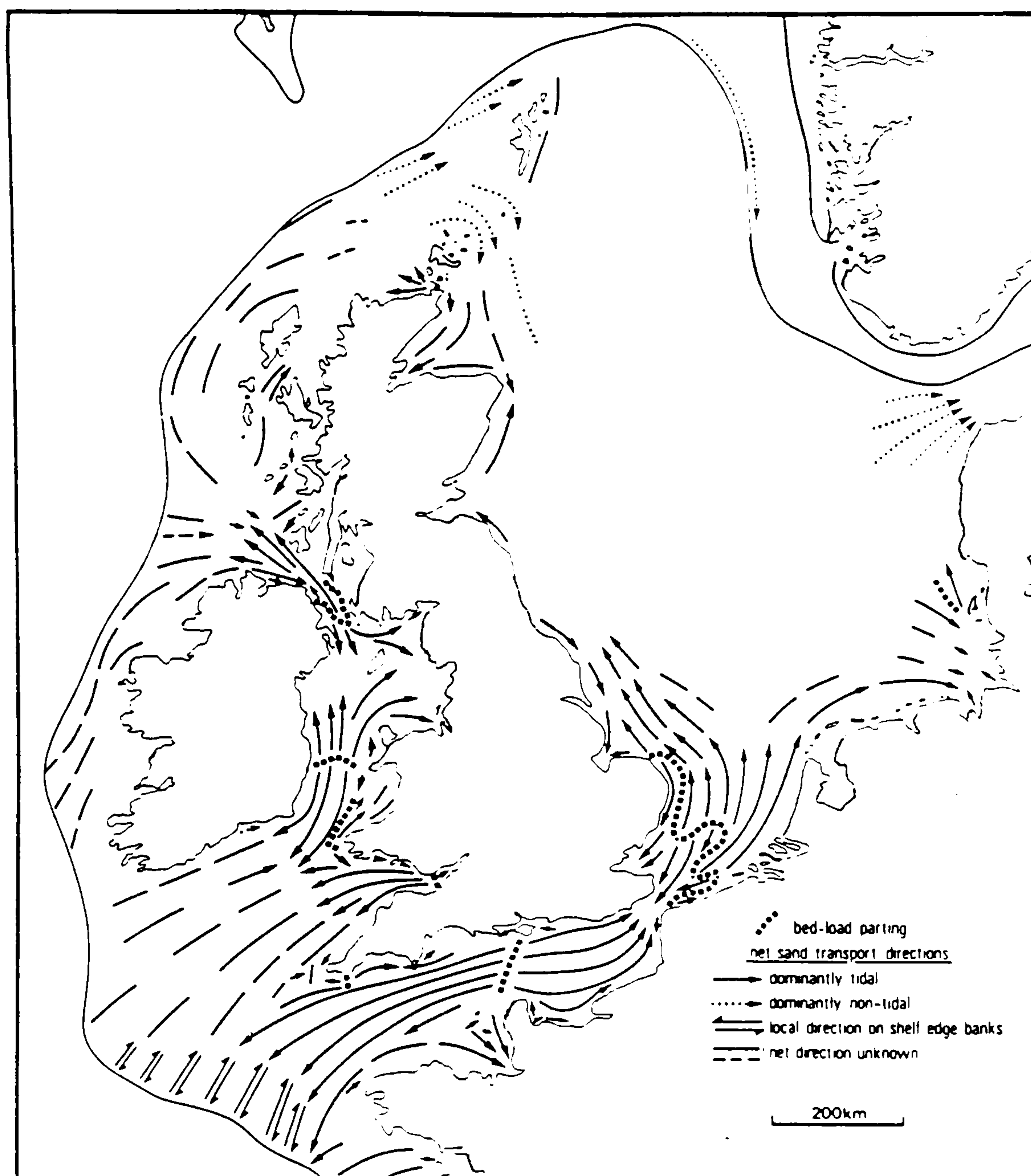
Figure 1.5: Net sand transport directions on the continental shelf around the British Isles [after Johnson et al. , 1982].
