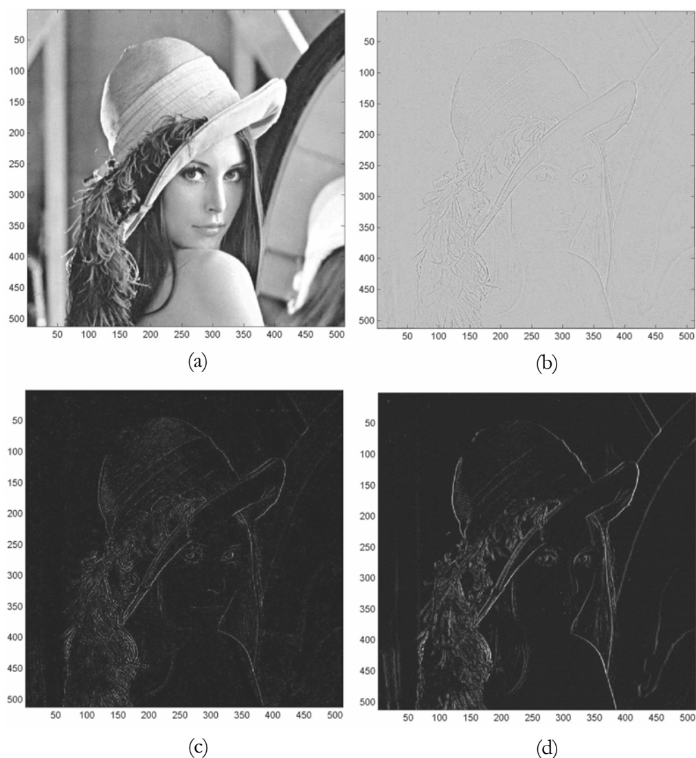
Figure 3-5 Activity marking: (a) Original image, (b) the result after Laplacian filtering, (c) the factor \alpha_{i,j} for "Edge marking" and (d) the factor \alpha_{i,j} for "Gradient marking"
