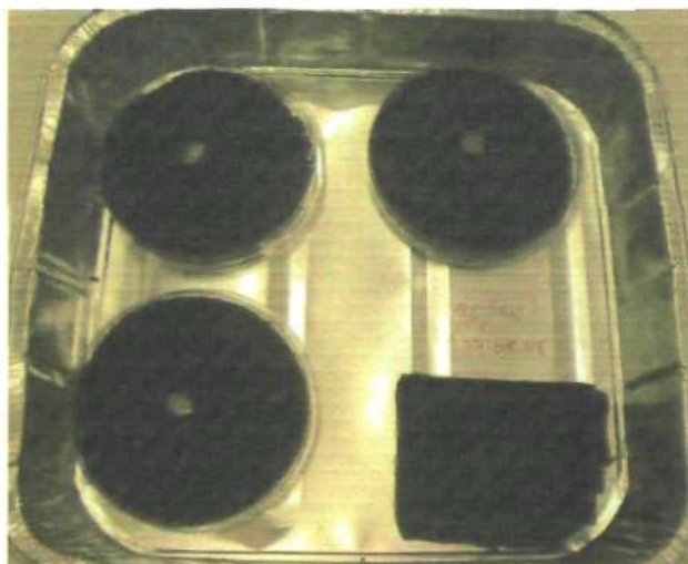
Figure 7c.1: Microcosm set-up – sieved soil added to empty sterile Petri dishes and inoculated with A. cylindrospora enriched with ^{13}\text{C} and ^{15}\text{N} at the central point of the dish.
