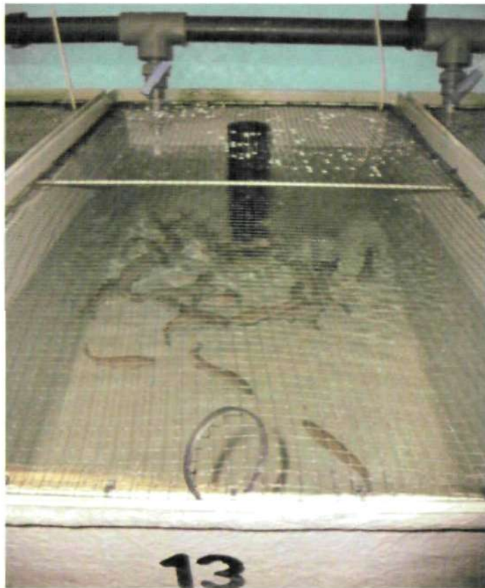
Plate 4-1: Recirculation system E at the University of Plymouth Fish Nutrition research unit. Note the fibreglass tanks, inlets and lights positioned above all the aquaria to ensure uniformity.
