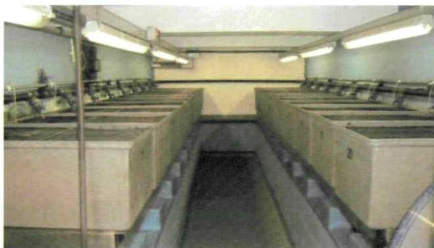
Plate 4-1: Recirculation system E at the University of Plymouth Fish Nutrition research unit. Note the fibreglass tanks, inlets and lights positioned above all the aquaria to ensure uniformity.
