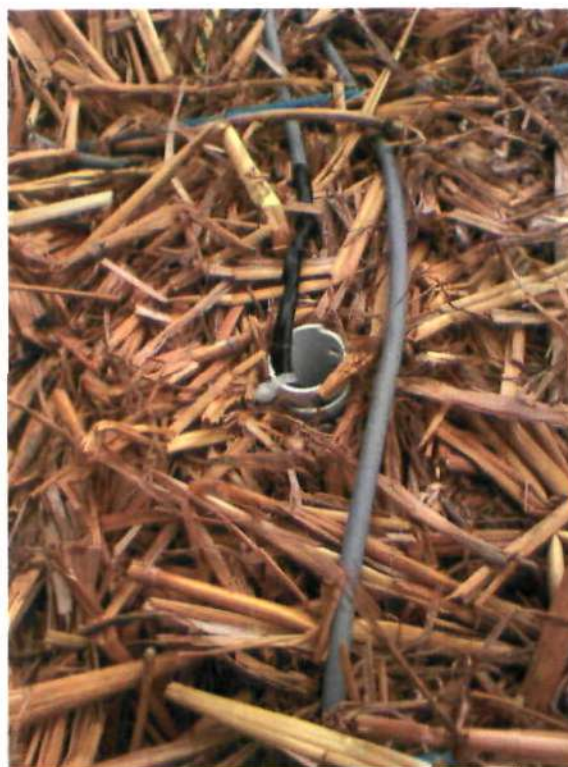
Fig.A13 RH and temperature sensors inserted into straw bale
