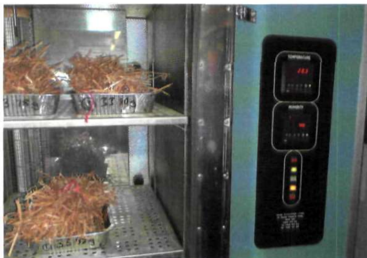
Fig.38 Samples of straw in the Environmental Chamber
