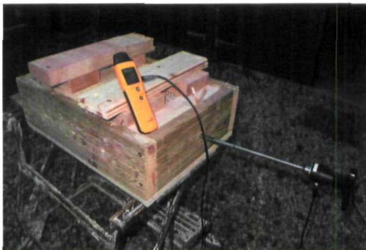
Fig.26 Box with straw fully compressed showing 'Balemaster' inserted
