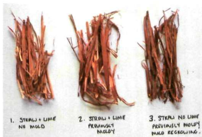
Fig.50 Three samples from desiccators at 97.3% RH
