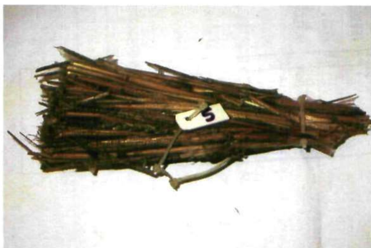
Fig.52 Sample of straw from desiccator at 98% from Lawrence (2009)
