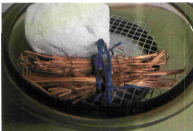
Fig.46 Desiccator containing two samples of straw with lump of plastered straw
