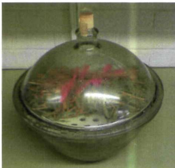
Fig.39 Sample of straw in desiccator at 97.42% RH
