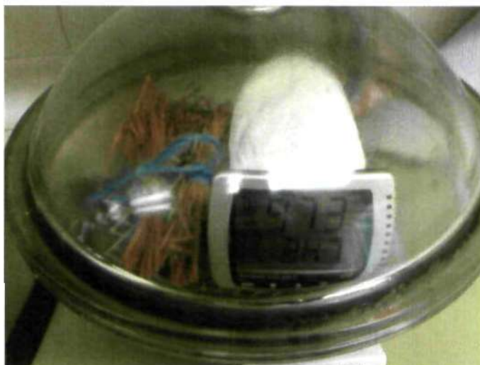
Fig.47 Straw samples in desiccator at 97.3% RH
