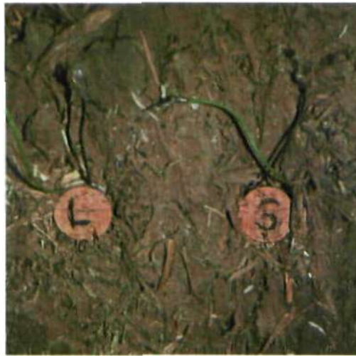
Fig.A24 Probes installed in earthen render
