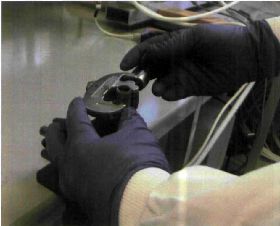
Figure 2.8 Use of rotating pipe cutter to cut samples for downstream processing.
