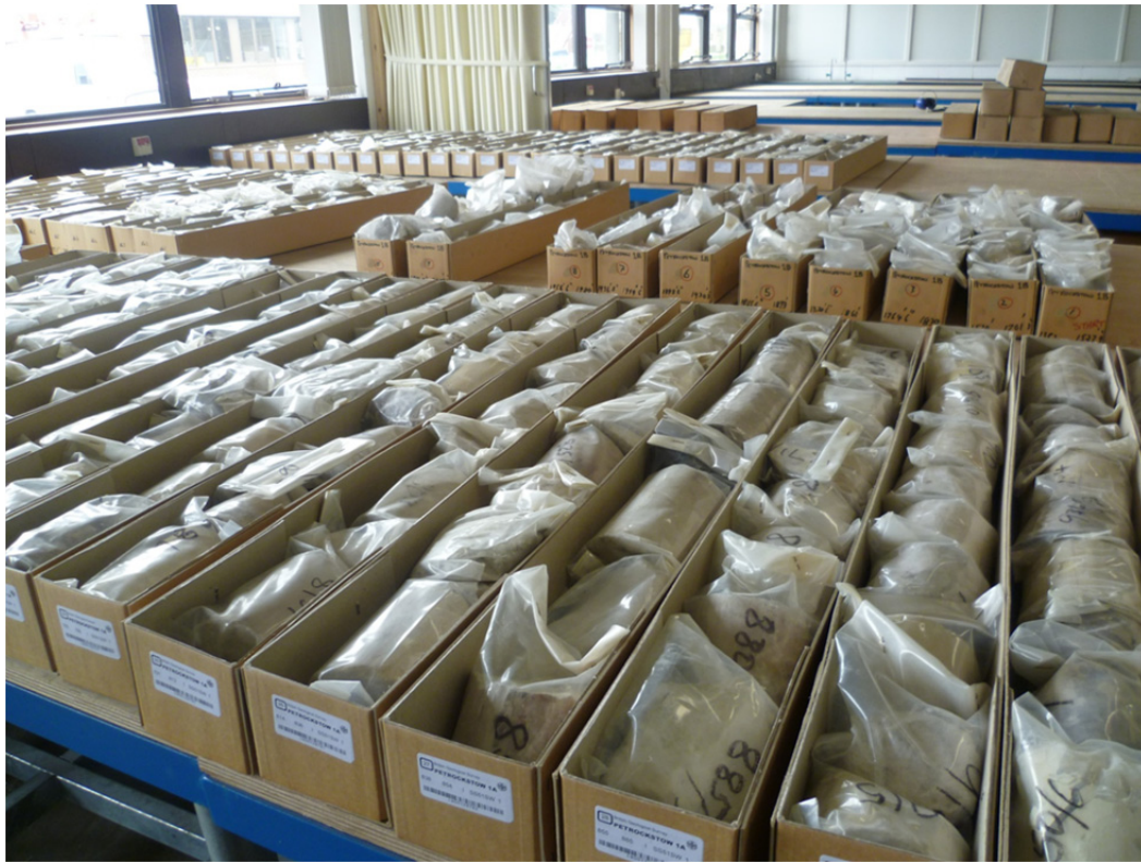
Figure 2.1: Petrockstowe core samples in the BGS Keyworth core laboratory displayed for description, logging and sampling by the Researcher
