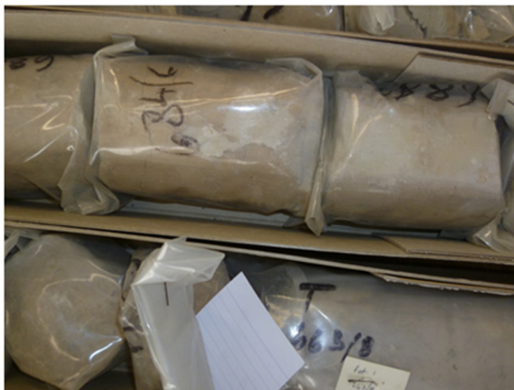
Figure 2.2: Part of a zoomed core sample (the cores are not slabbed) showing the condition of the core material at the GBS Keyworth, core laboratory
