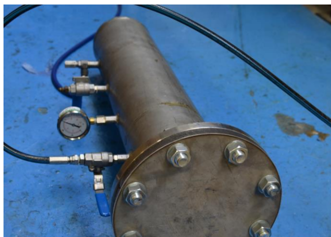
Figure 5.1 The hydrostatic chamber used in the diffusion test
