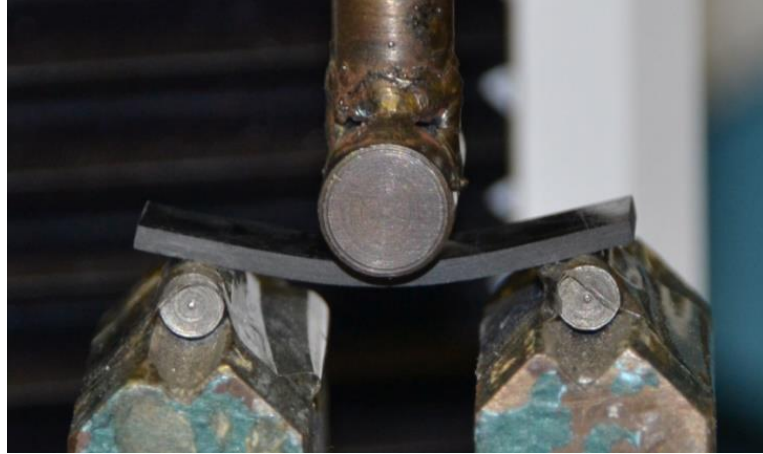
Figure 6.22 3-point bending creep test for the angle-ply laminate
