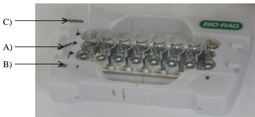
Figure 2-6: Loaded DG8™ cartridge for QX100 system. A) Center row for 20 \mu L PCR reaction. B) Bottom row for 70 \mu L of Droplet Generation Oil. C) Collection well for droplet generation.
