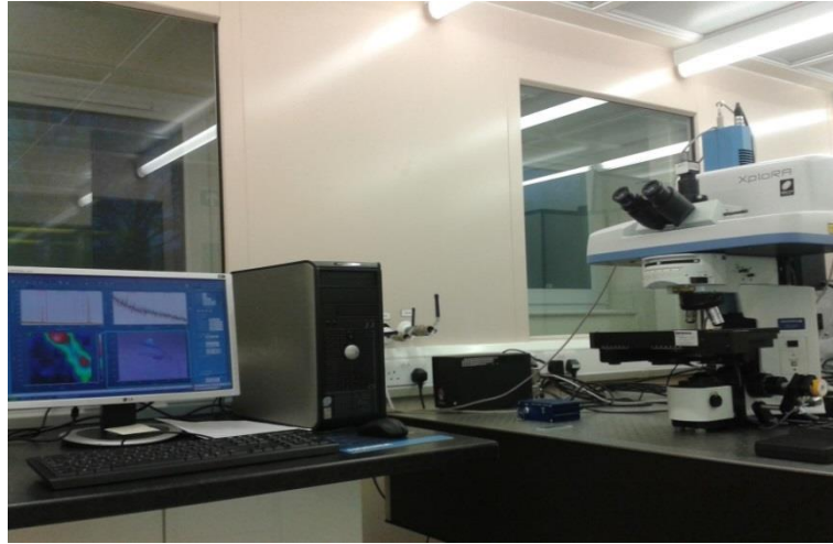
Figure 4-13. XPLORA Raman analysis system with an OLYMPUS BX41 microscope in Cleanroom (HORIBA, UK).
