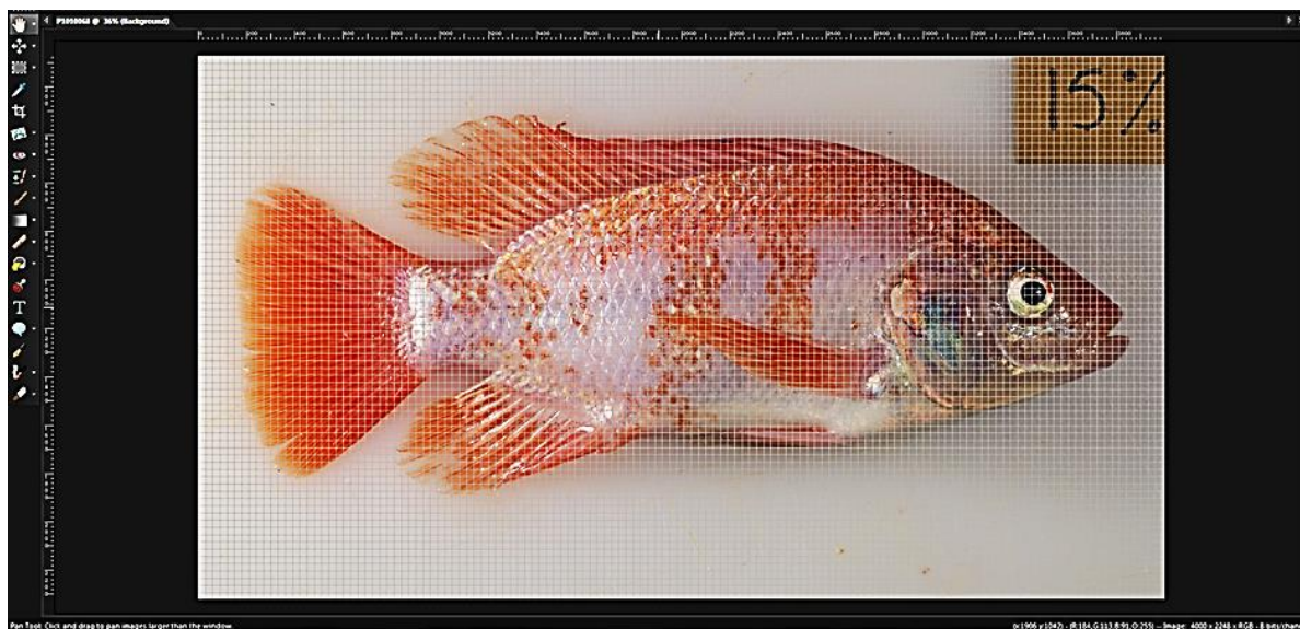
Figure 2.8 Example RAW image of fish from the 15% algal inclusion cohort analysed using Corel PaintShop Pro X4 with grid pattern superimposed for pixel analysis.
