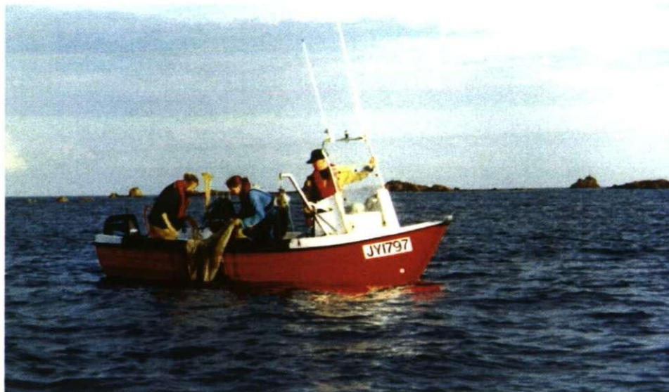
Figure 3.3 The small (5.5m) open boat with a 40HP 4-stroke petrol engine used in the deployment of trawl, pots and divers.
