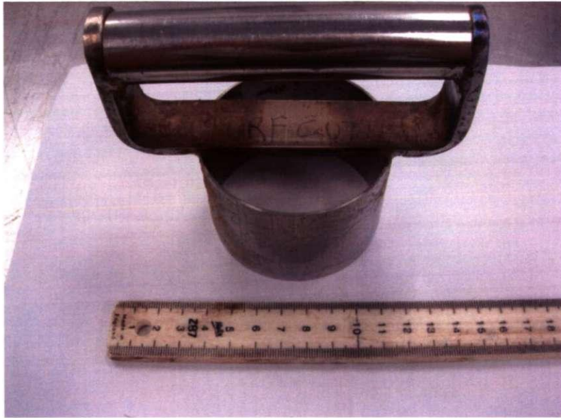
Figure 3.2 Hand-held sampler used to take the modern surface samples.
