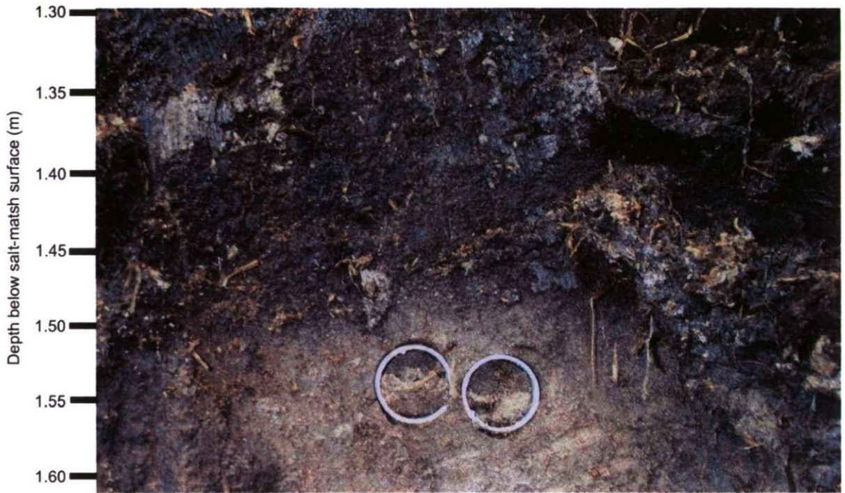
Figure 3.5. OSL sampling tubes in position in the cliff exposure at Oksby Enge (Sample number 4, Table 5.3).
