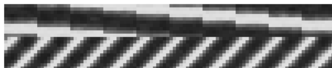
Fig. 8. Final u (y-axis) to v (x-axis) synaptic weights after training with 2-dimensional data (light represents a strong connection and dark represents a weak connection; the top half of the graphic is the bank of input neurons encoding the first dimension and the bottom half is the bank encoding the second dimension; and each ten steps along the x-axis represents a row of output neurons, then the next ten represent the next adjacent row, and so on): the connections to the output layer vary in one dimension across an individual row (with consistency throughout the map), and vary in the other dimension across the rows, encoding the current input as a location in the output map in an organised way. A change in one input dimension (the bottom 10 rows) as one moves through each row of the output layer (each block of 10 columns), and a change in the second dimension (the top 10 rows) as one moves down through rows in the output layer (changes between each block of 10 columns in the figure) can be seen. For a given output neuron (one column), a gradual decrease in weights either side of a central point in each input dimension is visible.
