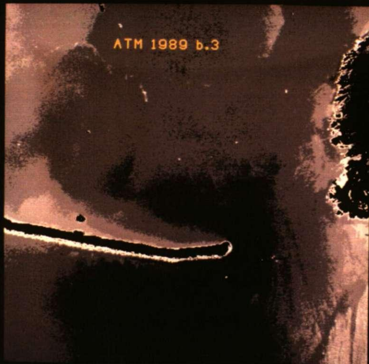
Figure 6.29 ATM 1989 Low Water contrast stretched band 3 image of the Eastern Entrance (520-600nm).
