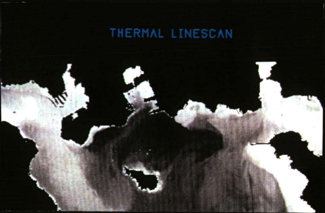
Figure 6.15 Daedalus AADS 1230 a geometrically corrected and contrast stretched thermal image of the Hamoaze Channel.
