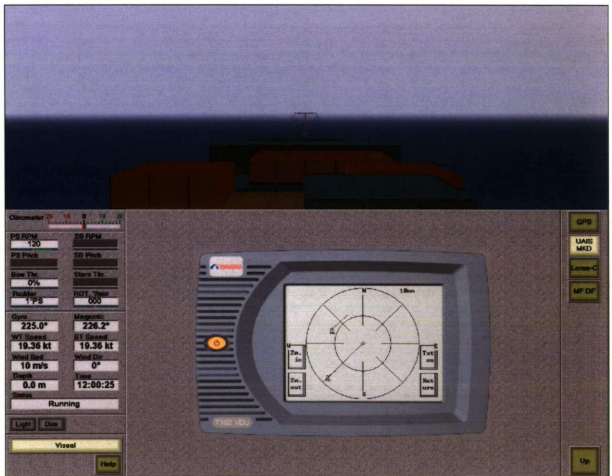
Figure 5-1 TRANSAS AIS MKD on the main console
