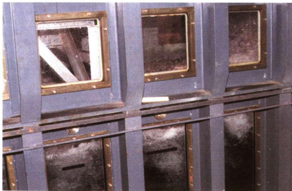
Figure C 6. Rig Operating with Hood in Place (Operation is at high load; aeration of water and associated rise of water level above the static value (black mark) can be seen).
