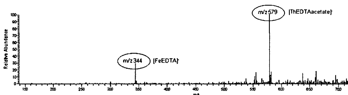
Figure 3.4 Example electrospray ionisation mass spectrum showing aqueous complexes of [\text{ThEDTAacetate}]^- ( m/z 579) and [\text{FeEDTA}]^- ( m/z 344) from a sample of 420 \pm 30 \mu\text{M} Th pre-equilibrated for 48 h with 420 \mu\text{M} EDTA before the addition of 800 \mu\text{M} Fe, in 0.05 \text{ M} ammonium acetate after 49 days
