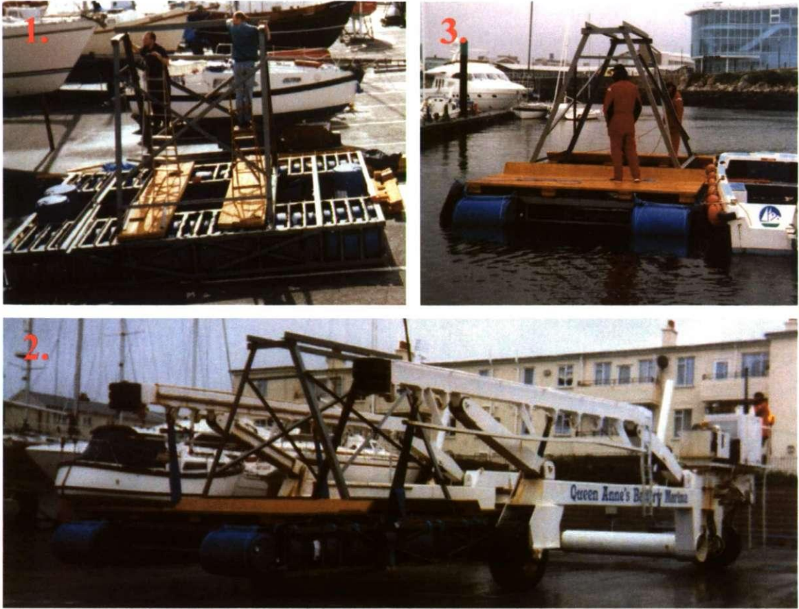
Plate 3.5 Views of the UOP research pontoon R.P. AMAP-1 during: (1) fabrication at Queen Anne's Battery Marina, (2) prepared for its maiden launch from a mobile cradle, and (3) being moved to a berthing awaiting towage to Calstock (note the shallow draught of the pontoon).
