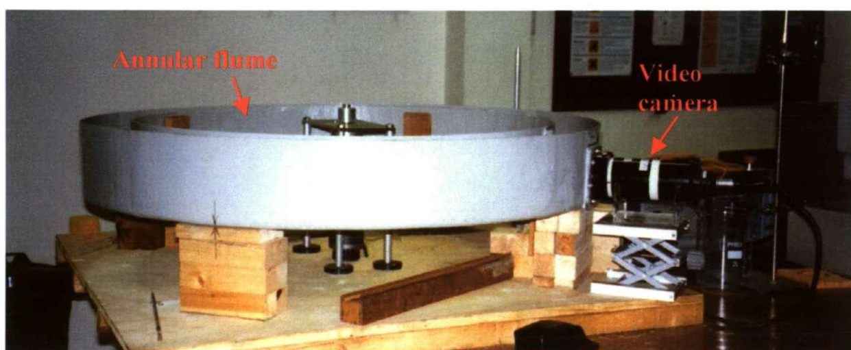
Plate 3.13 UOP annular flume (with rotating roof section removed) with the video camera inset into the flume wall.
