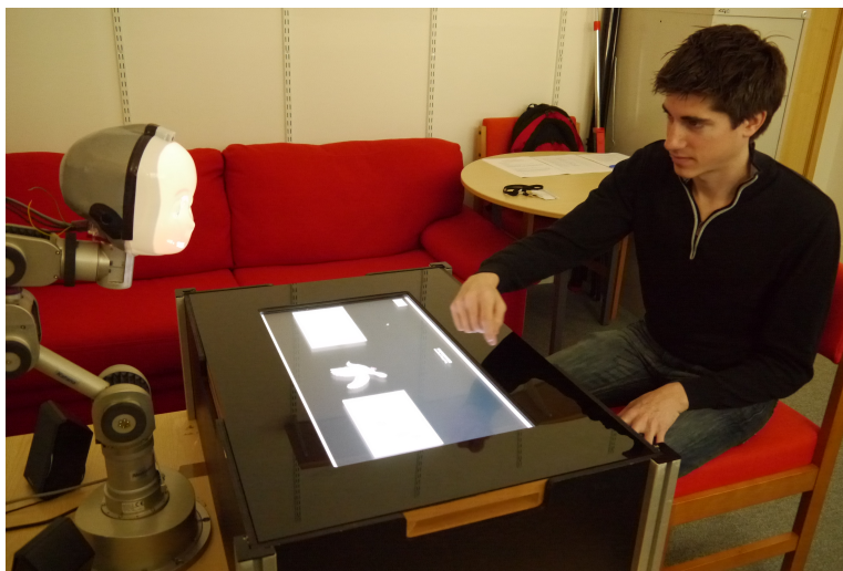
Figure 5.2: Experimental setup: the participant faced the LightHead robot; both shared the context procured by the touch-screen.
