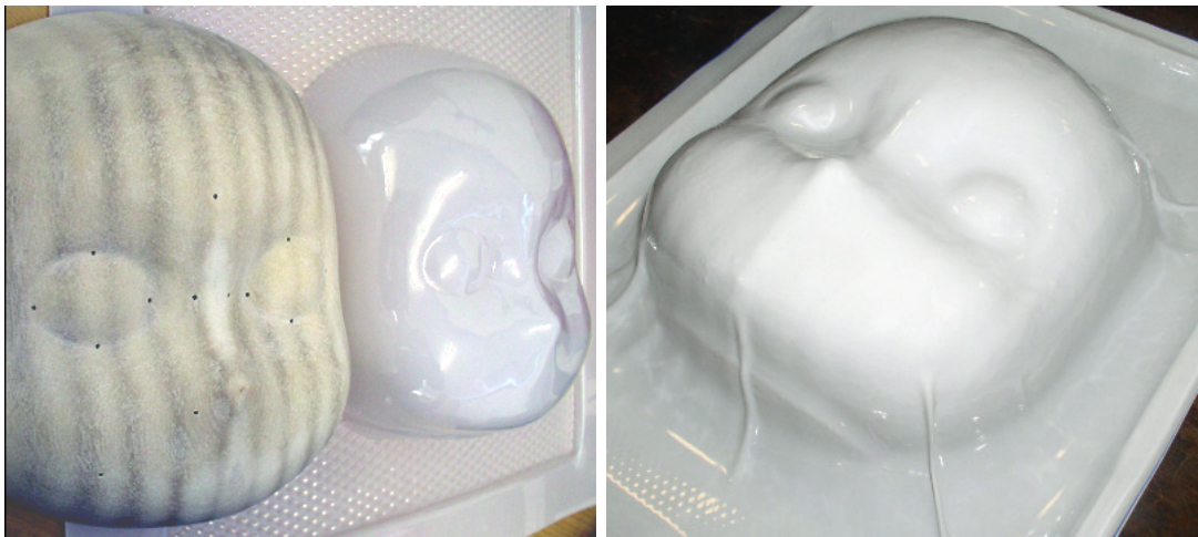
Figure 3.3: Left: mould and mask. The mould requires sanding to smooth the layers still visible and drilling in the ridged areas (e.g. eye sockets); this prevents trapping air pockets so the vacuum process correctly shapes these areas. Right: foldings can appear if the temperature for vacuum forming is too high or the plastic too thin.
