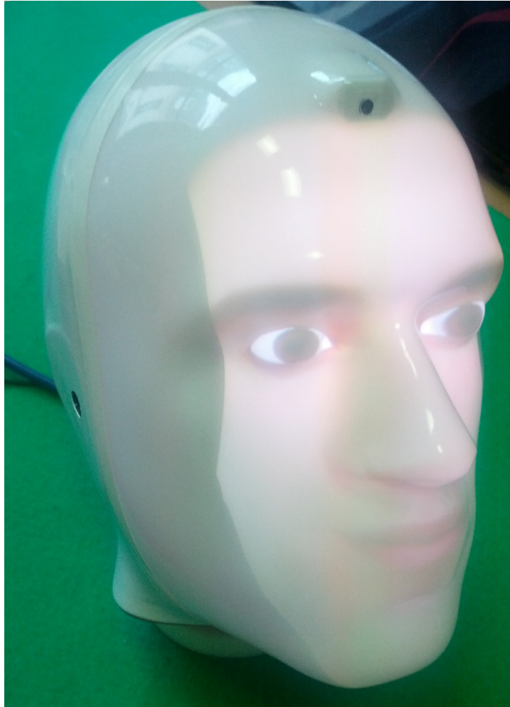
Figure 7.2: The Lighty prototype as commercialized by the spin-off Synthelligence until 2015 7 . Projected face, form-factor and some materials have been updated compared to LightHead v4.
