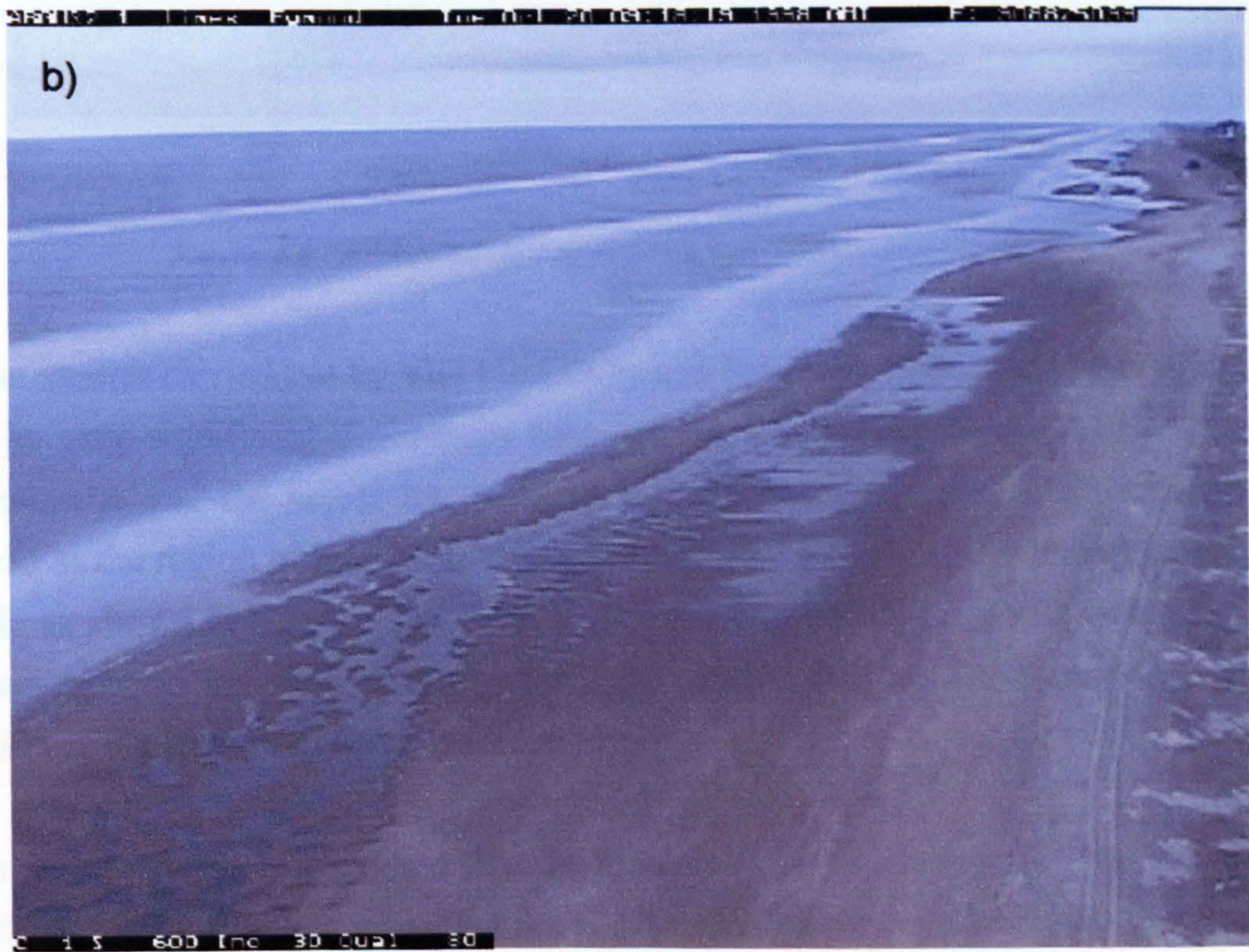
Figure 4.8 Argus video image showing wave breaking intensity patterns over submerged sandbars at Egmond aan Zee, Netherlands. (a) snapshot, (b) 10 minute time average.
