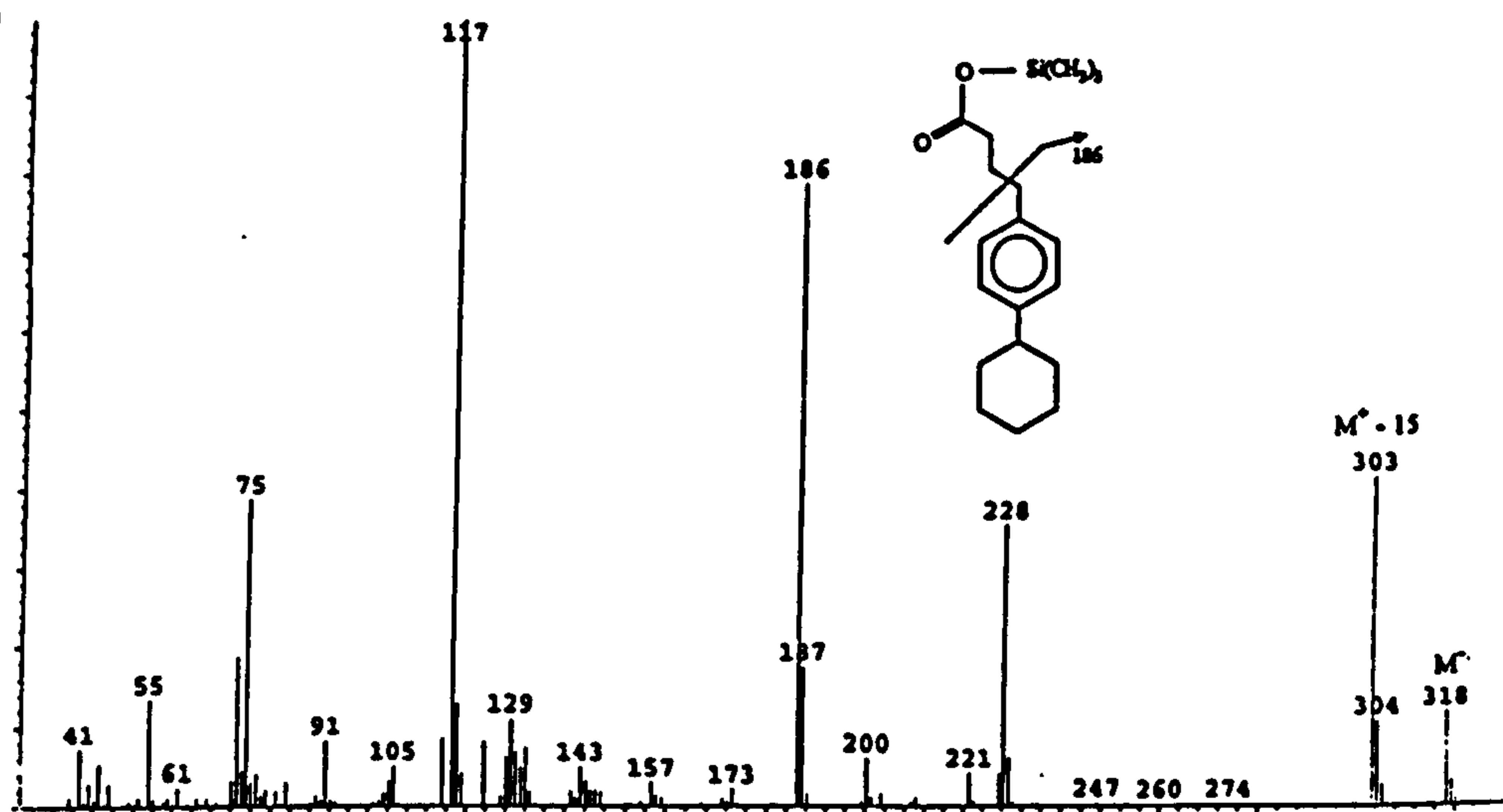
Figure 3.17 Cont'd Mass spectra of principal components of the total organic reaction products (derivatised with BSTFA) from alkylation of phenylcyclohexane using \gamma -butyrolactone
