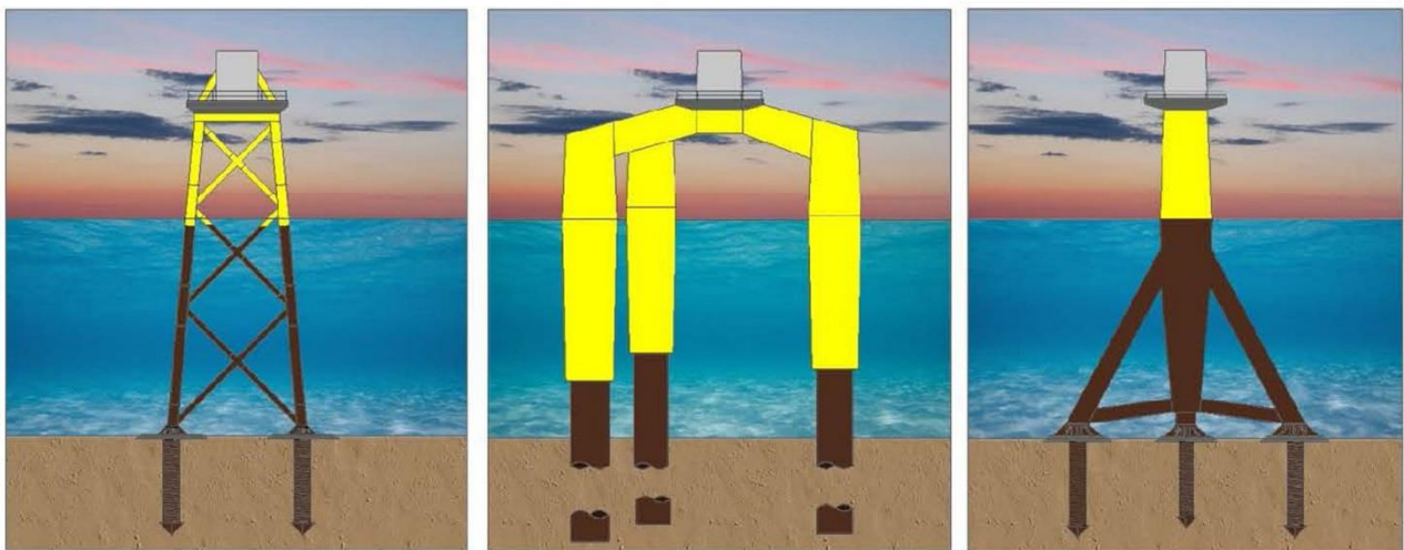
Figure 10: Transition water substructures: from left to right, jacket frame, tri-pile and tripod
