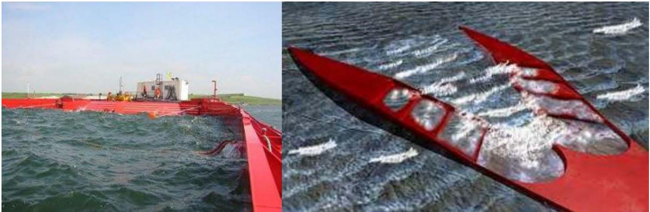
Figure 14: Examples of overtopping converters: WaveDragon, left (courtesy of Wave Dragon AS, left[98]) and WaveCat, right (courtesy of the COAST Research Group at Plymouth University [99], [100])
