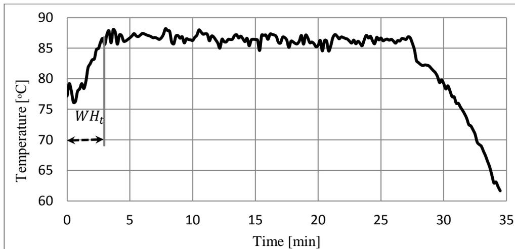
**Figure 12** Temperature of the hot water at the inlet during tool heating.
