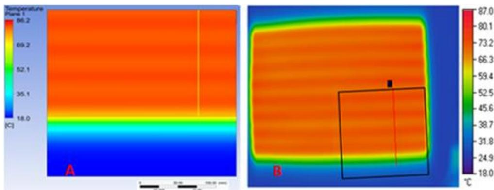
**Figure 16** Numerical and experimental thermal images of the tool surface at the corresponding heating times. **A:** quarter of the tool model surface, numerically. **B:** total tool surface, experimentally by thermal camera.
