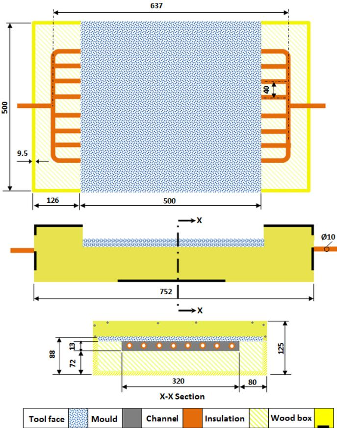
Figure 1 Dimensions (mm) of the optimal experimental tool
