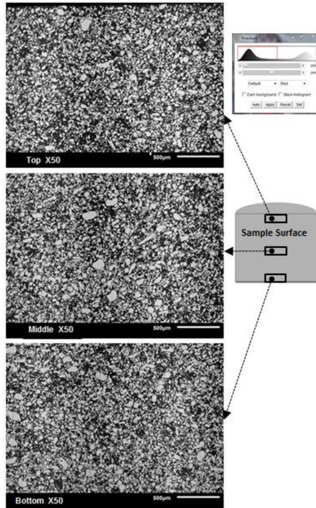
**Figure 4** Aluminium particle concentration in the Alepoxy mixture, magnification is X50
