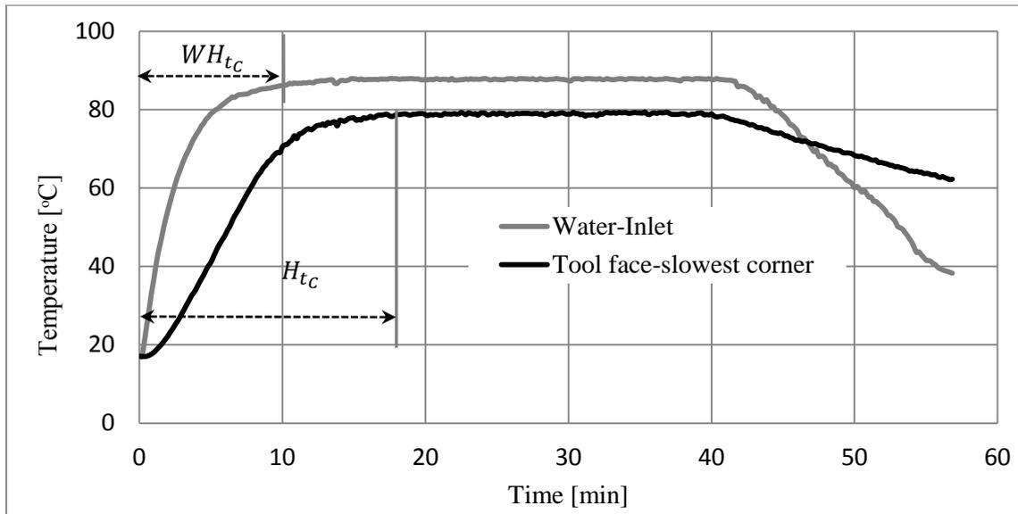
**Figure 11** Temperature curves during heating of the cold water and tool.
