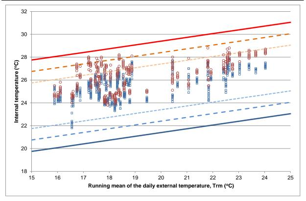
Figure 1 BSEN15251 thresholds and the hourly temperatures measured in the living room and bedroom of House 2 (Code for
